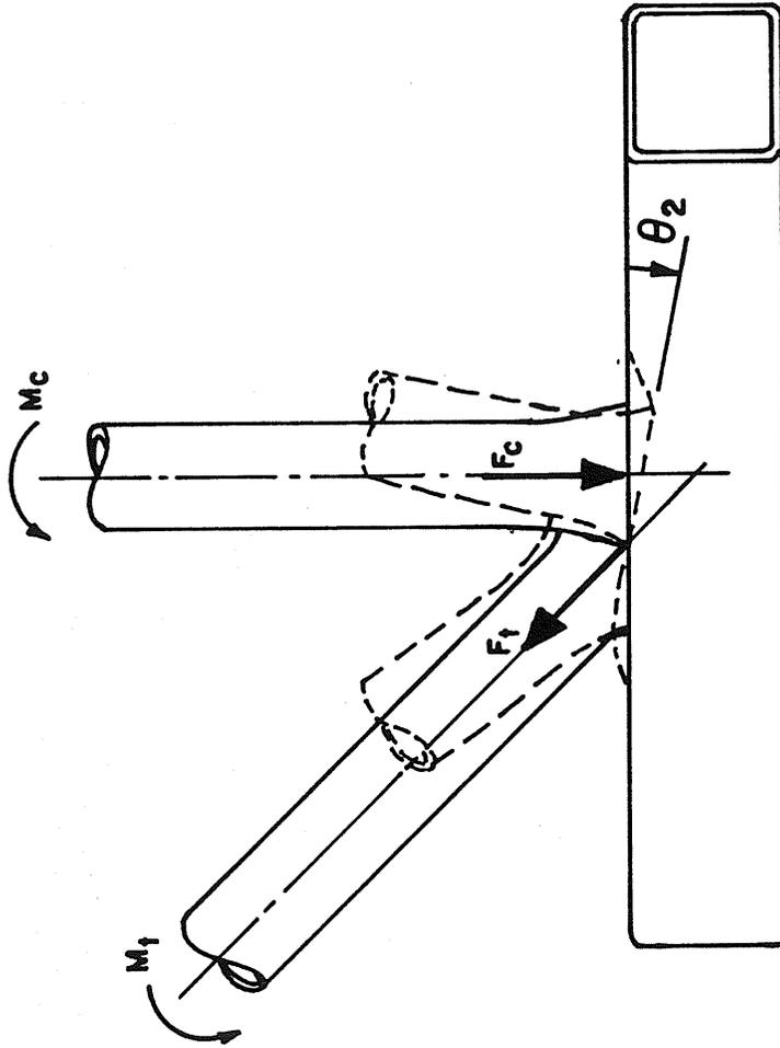
FIG. 4.3 FAILURE MECHANISM
