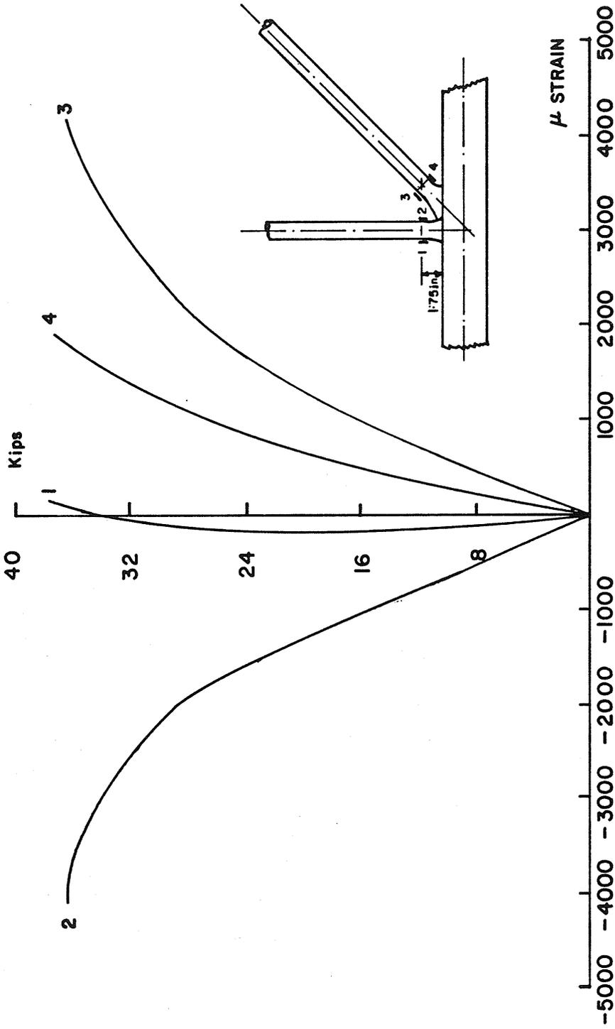
FIG. 4.6(a) STRAIN PLOTS, JOINT 4A50, TRUSS-1
