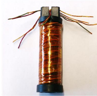
Figure 2: Bobbin with wires pulled back.
