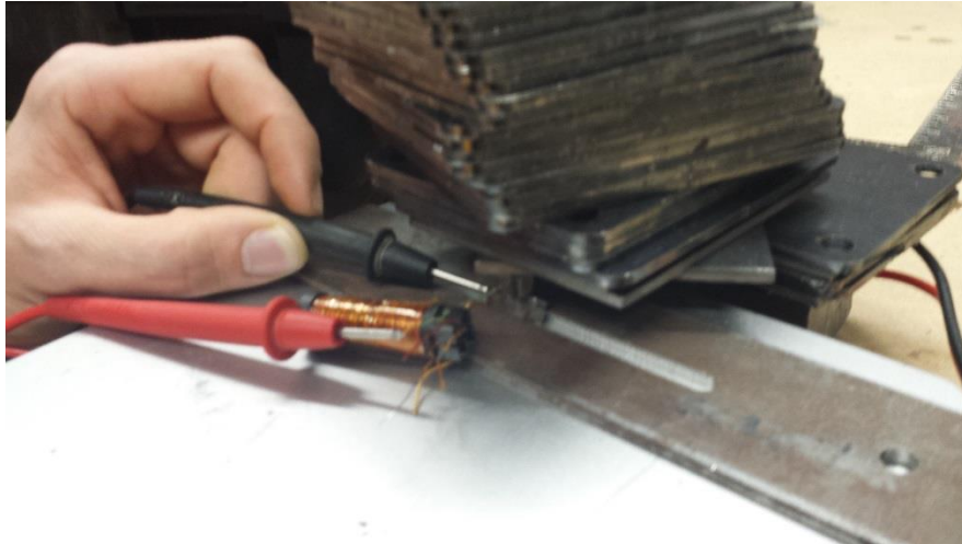
Figure 2: Photo of apparatus setup showing multimeter test lead connections to bobbin wire and tool steel bit.
