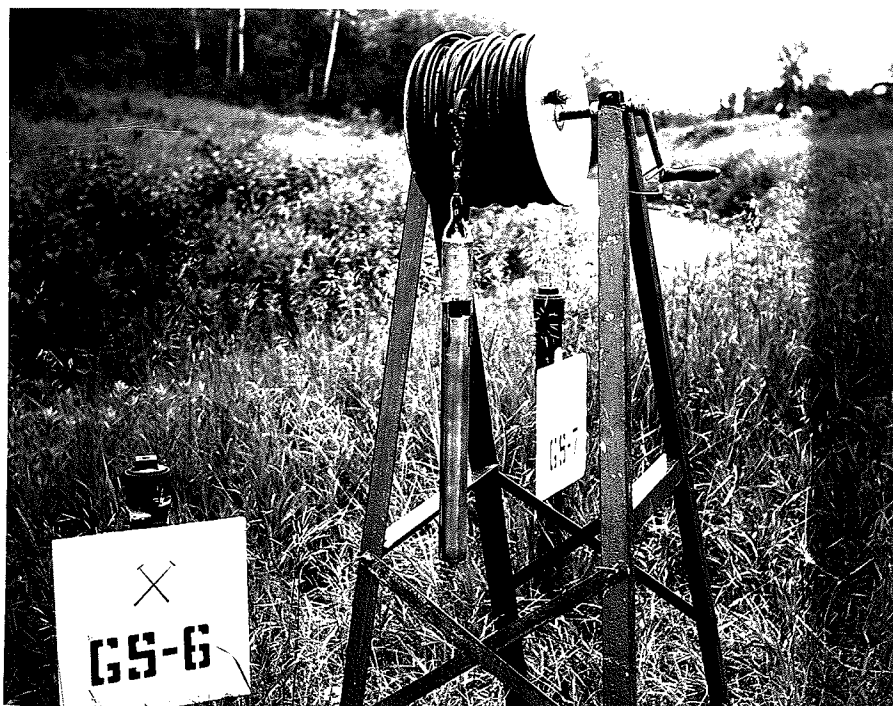
Fig. 38 - The deep piezometer sampler.
