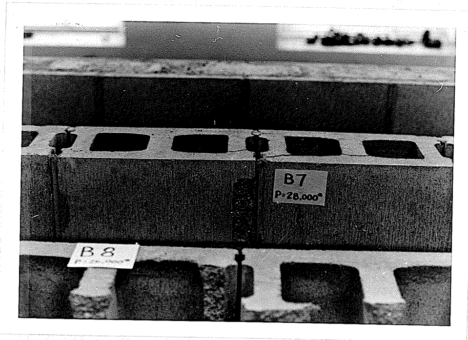
FIG. 48 BEAM 7 - FLEXURAL FAILURE BY CRUSHING OF BLOCKS
