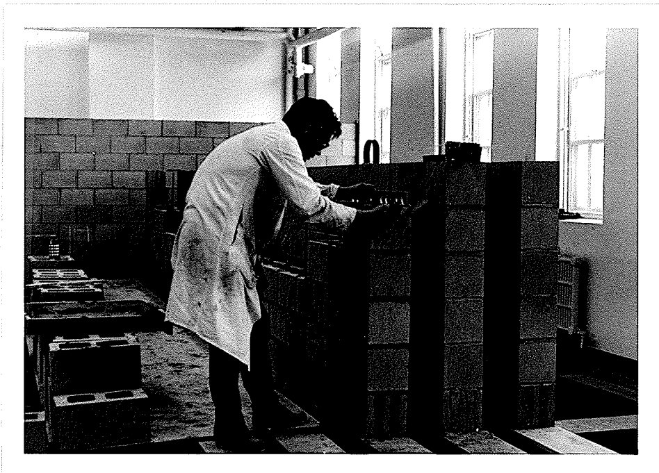
FIG. 14 METHOD OF LEVELLING END BLOCKS
