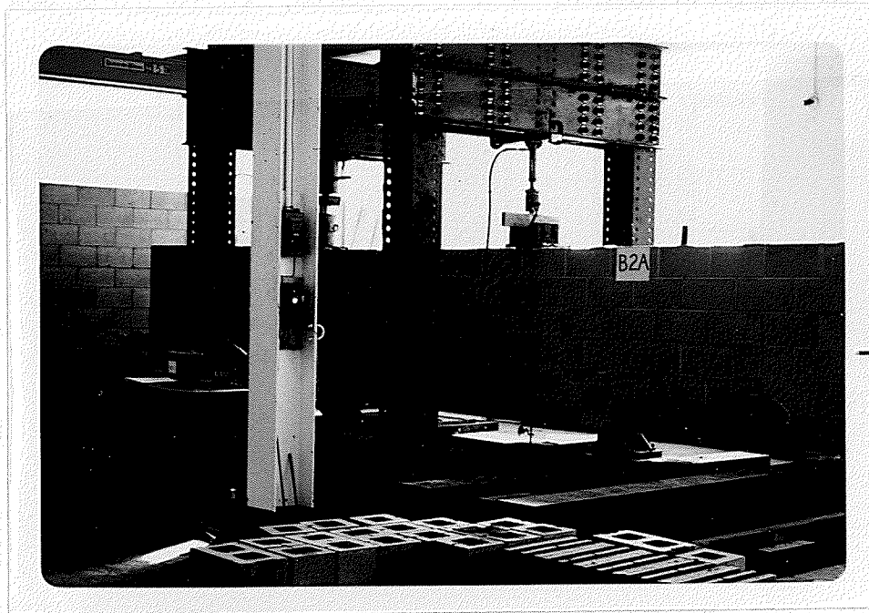
FIG. 29 MASONRY BEAM IN TESTING POSITION
