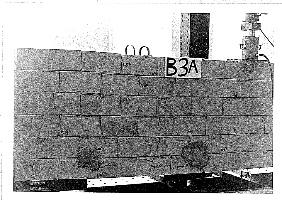
FIG. 39 SHEAR FAILURE IN BEAM 3A
