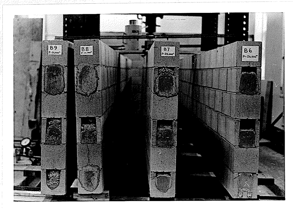
FIG. 52 POOR QUALITY CONCRETE IN RIGHT END OF SERIES 2 BEAMS
