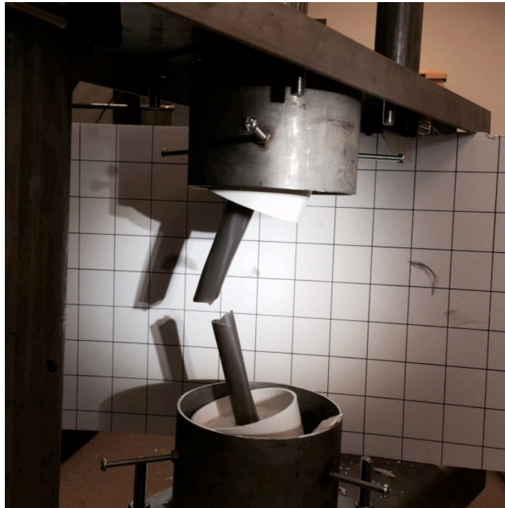
Figure 24: Orientation of the PVC pipe couplings after bone specimen fracture
