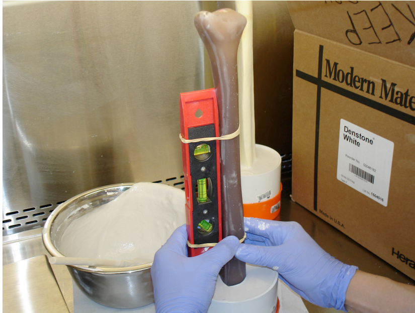
Figure 5: The cementing process of the composite tibia specimen
