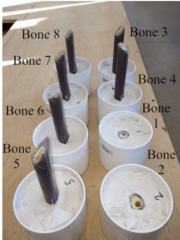
Figure 23: Inferior portions of the composite bone specimens after fracture
