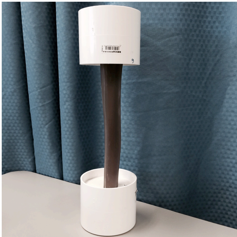
Figure 6: A composite tibia specimen prepared for testing
