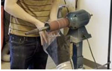
Figure A14 - Grinder smoothing trim lines
