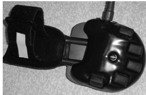
This is a picture of the hand held response pad. The Velcro strap keeps it on the arm while fingers are free to press the buttons in response to questions.
