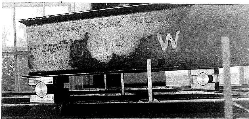
Photo 11. Attachment of measuring scales for checking deflections.
