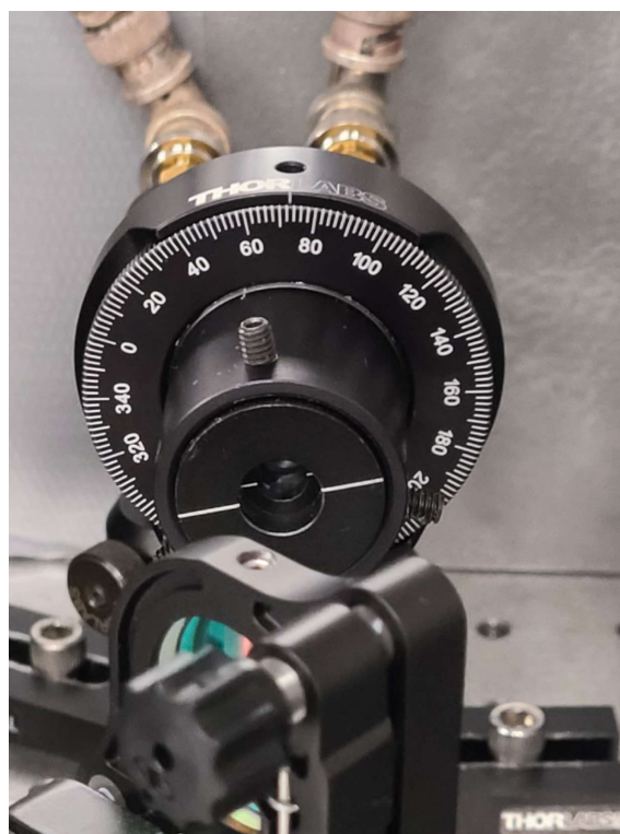
Figure 3.16: An image of the Wollaston prism used for the majority of this project
