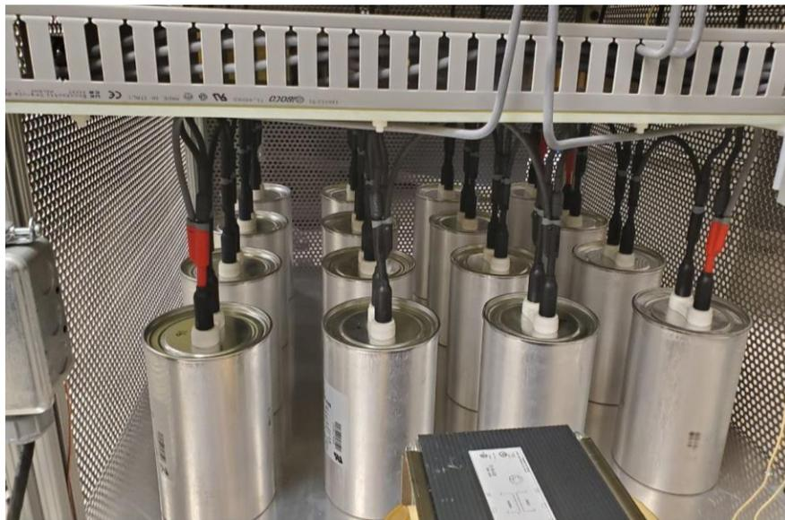
Figure 5.3: The capacitor ladder implemented in the prototyped CL-EVR [83-84].
