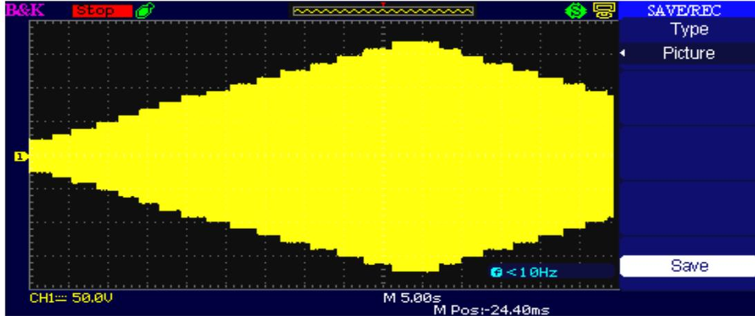
Figure 5.26: The voltage across the resistive load up-stepped from level 1 to 16 and subsequently down-stepped from level 16 to 8.
