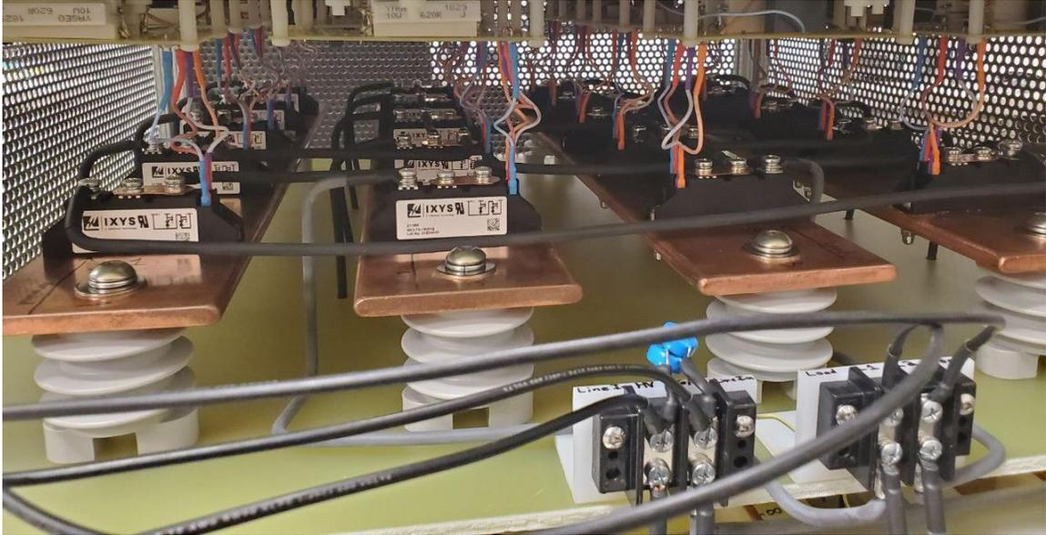
Figure 5.4: The TRIAC implemented in the prototyped CL-EVR [83-84].
