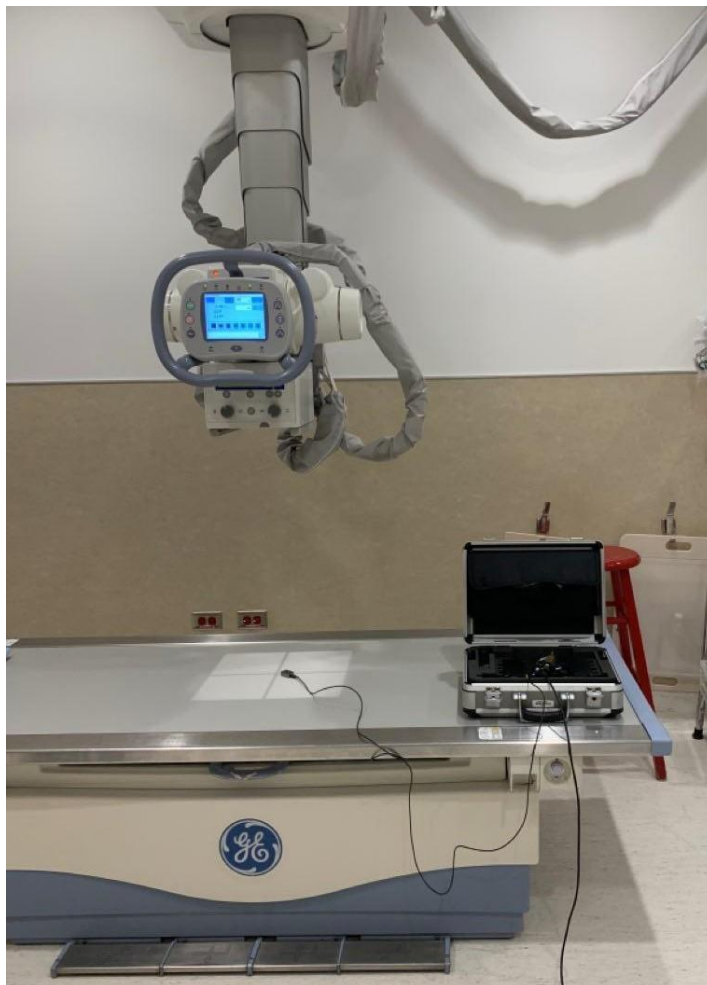
Figure 3-1. The setup used for measurement of accuracy of tube voltage, time-current product and exposure.
