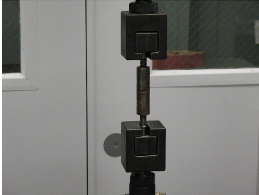
Figure 3-3 Typical thermal spray bond test set-up
