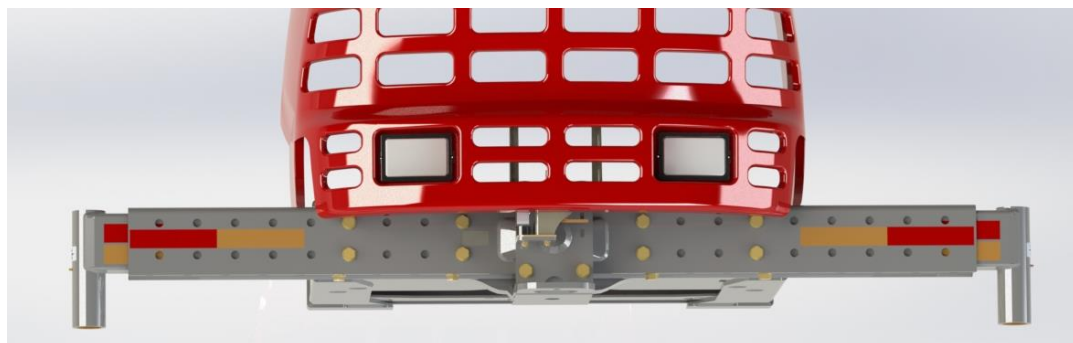
Figure 12: Rendered image of the rear of the tractor, showing the 8 axle bolts.
