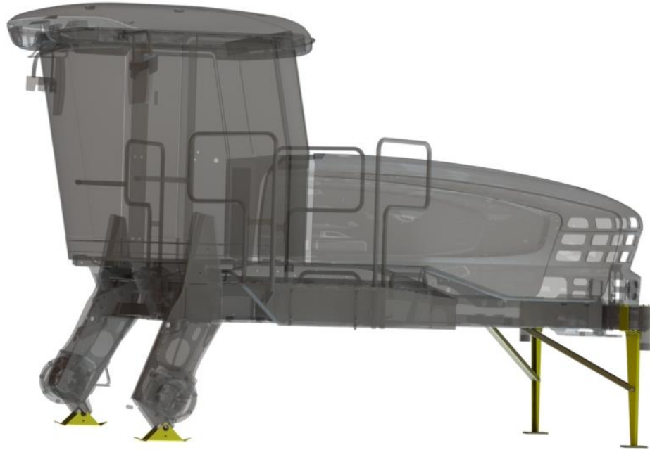
Figure 7: Final stand assembly (yellow components) shown mounted to a tractor.
