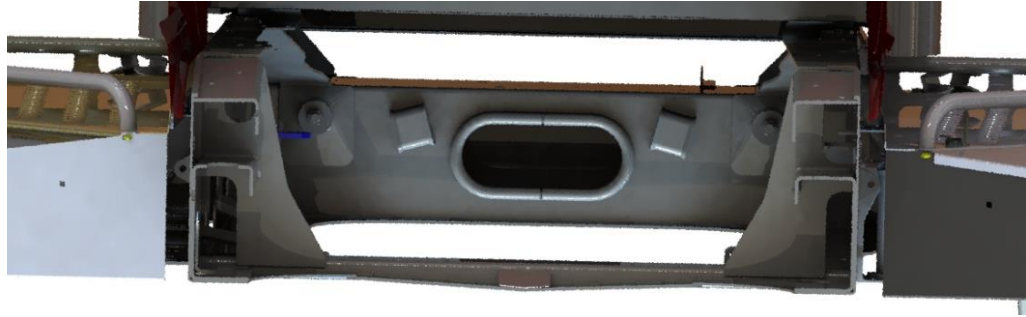
Figure 46: Cross sectional view of the tractor frame showing the cross member (bottom of image) that is not in the level plane as the rest of the frame.
