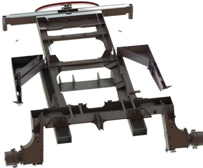
Figure 58: Cross sectional view of the tractor frame showing how the attachment fits with the frame.
