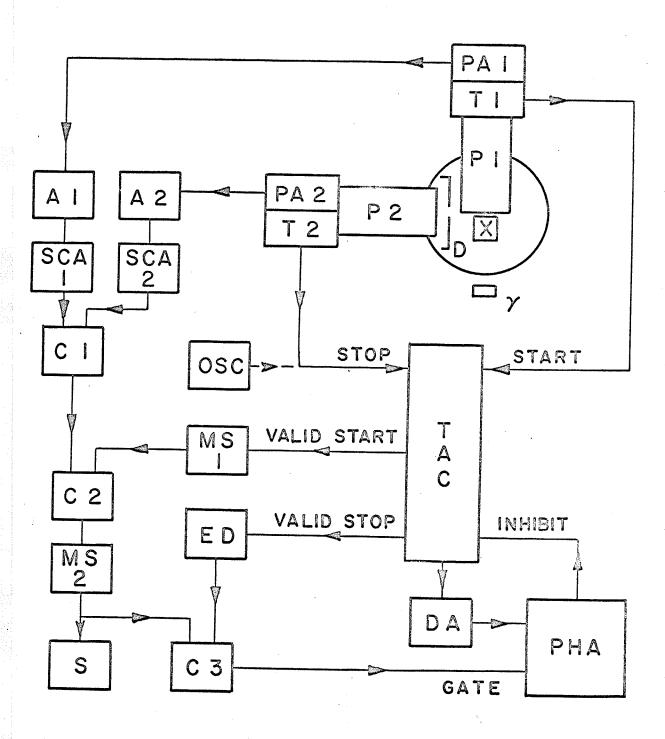
The time interval between the signals from Tl and T2 is converted into an analogue voltage pulse by the time-to-amplitude converter (TAC). This pulse is transmitted via a two microsecond delayed amplifier (DA) to a pulse height analyser (PHA) for possible storage.
