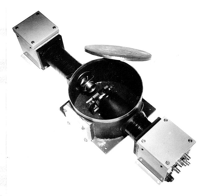
chamber itself, is enclosed in a box, insulated with four inches of polyurethane foam. A control system was designed to maintain the temperature of the box interior constant to within  $\pm$  0.5°C for temperature other than ambient room.
