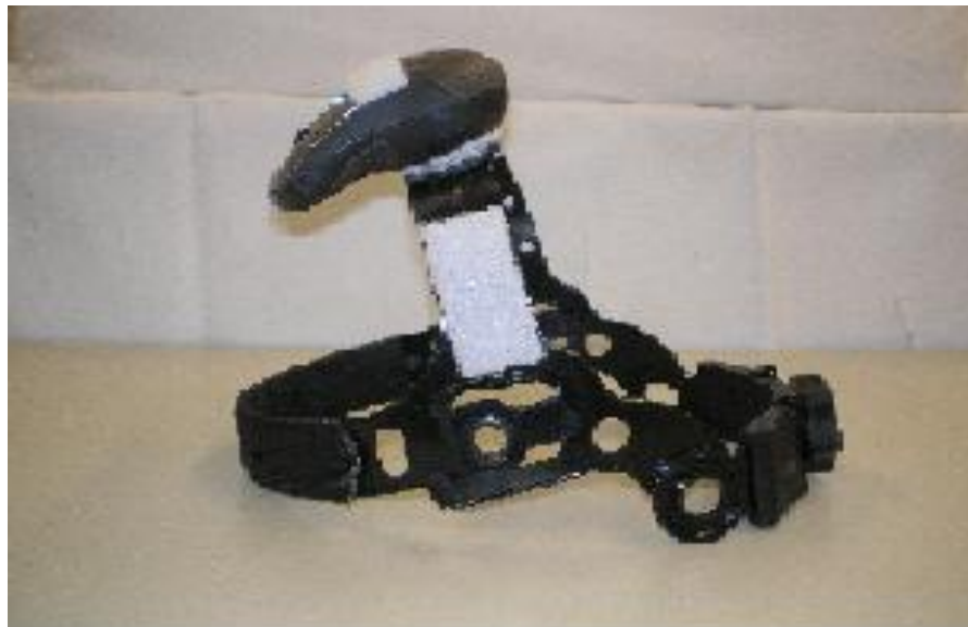
Figure 5: Head mounted air mouse on frame worn on head to move paddle or game sprite
