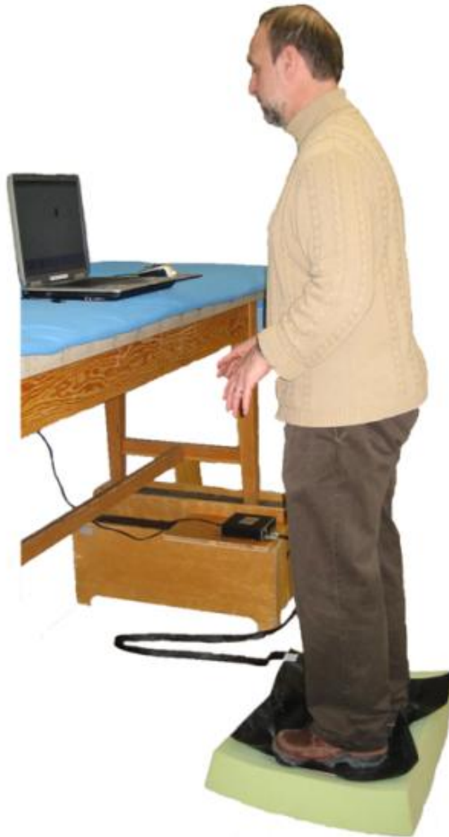
Figure 3: FSA pressure mat on top of sponge attached to FSA interface
