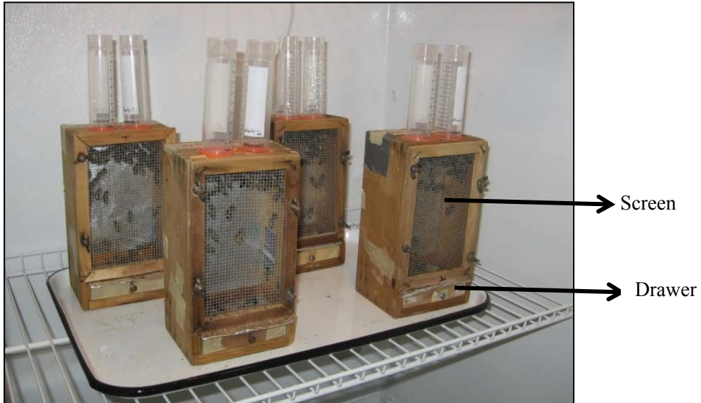
Figure 4.1. Wooden bioassay cages used for the grooming experiments. Below each cage is a screened floor with a drawer that allows fallen mites to be removed from the cage.
