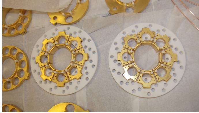
Figure 5.6: An 8-segmented electrode (octopole) was included with the intention of using it for rotating-wall compression of ions. However, many segments have now been shorted to reduce the complexity of the electrical connections and feed-throughs, making quadrupoles the highest order trap electrode configuration currently in use.
