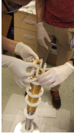
Figure 5.18: Electrodes within CPET were reconfigured and/or shorted to minimize the possibility of Penning discharges.
