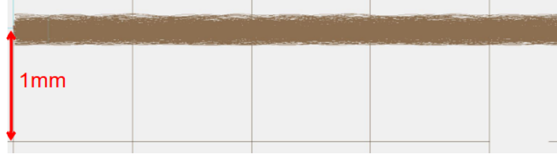
Figure 5.25: SIMION simulations of the ion radius inside CPET upon injection without using the second ion source steering element (IS S2) to apply focal corrections to the beam. The radius could be kept as small as \sim 0.2 mm with these injection settings (sagittal view).
