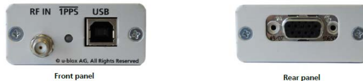
Fig. 6-13 - Front and rear panels of the GPS unit
