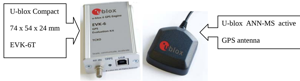
Fig. 6-12 - GPS unit: EVK-6T-0 u-blox 6 Evaluation Kit with Precision Timing
