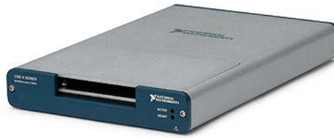
Fig. 6-10 - Multifunction Data Acquisition hardware NI USB-6361 from National Instruments
