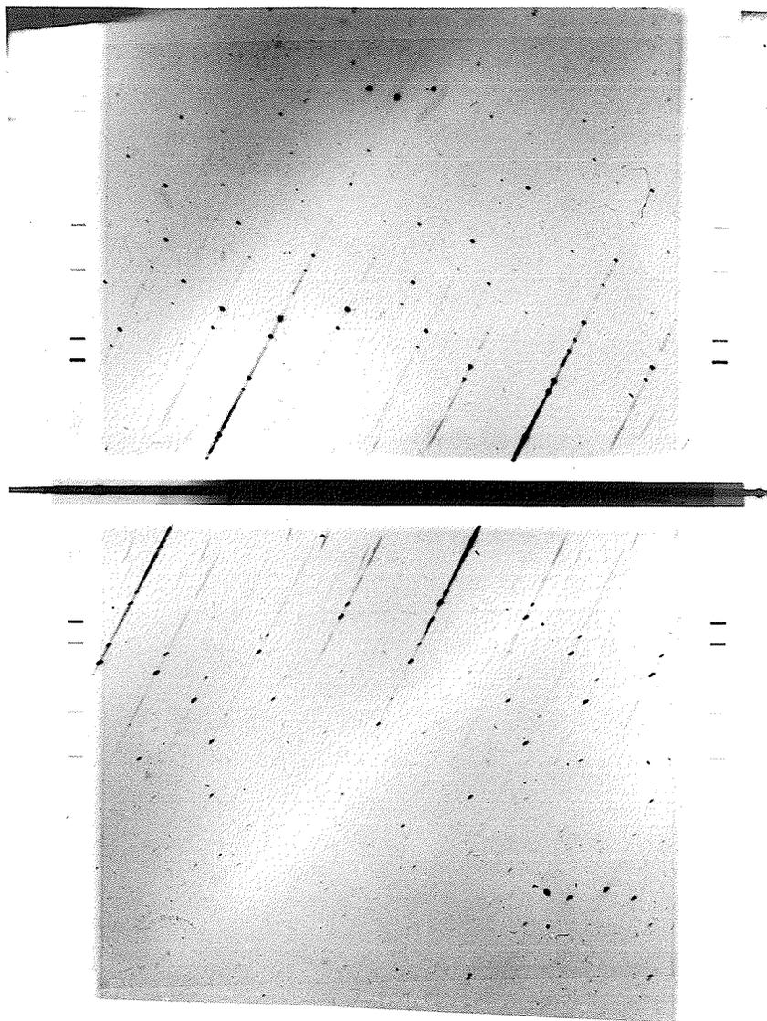
Fig. 29.  $hk0$  Weissberg photograph, Cu/- radiation; aluminum powder pattern, Cu/Ni radiation; camera radius 28.648 mm.
