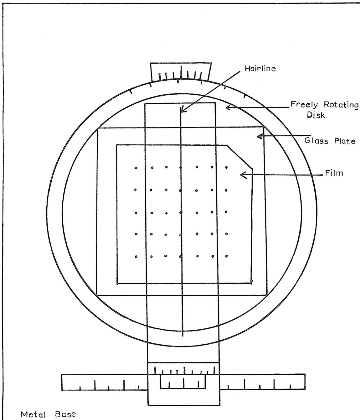
Fig. 7 Measuring device for X-ray photographs.
