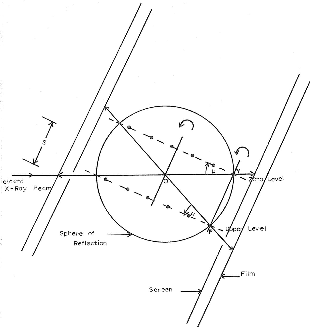
Fig. 11 Experimental arrangement for the equi-inclination Weissenberg method.
