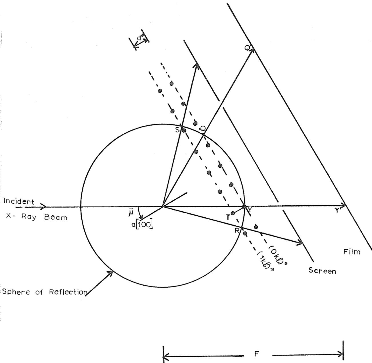
Fig. 4. Experimental arrangement for the precession method.
