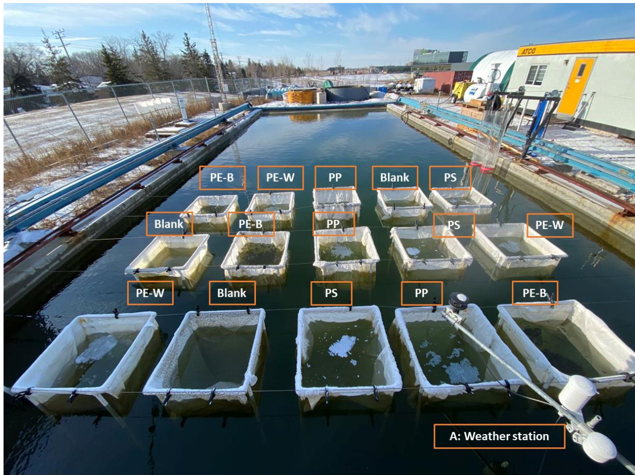
Figure 2-1. The set-up of the mesocosm experiment with 15 microcosms at the Sea-ice Environmental Research Facility (SERF) of the University of Manitoba, Winnipeg, Canada. PE-W: white color polyethylene; PE-B: black color polyethylene; PS: polystyrene; PP: polypropylene; A: weather station.
