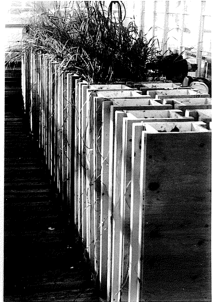
Fig. 3.4.7 Arrangement of the soil columns in the greenhouse.
