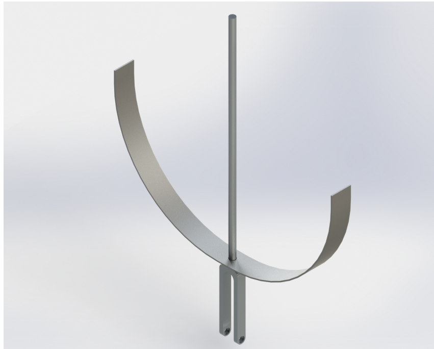
Figure 19: Nose Gear Concept 5 | U-Flex plate concept render
