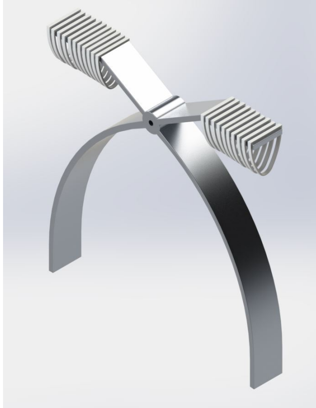
Figure 12: Main Landing Gear Concept 3 | Rubber Elastic Springs
