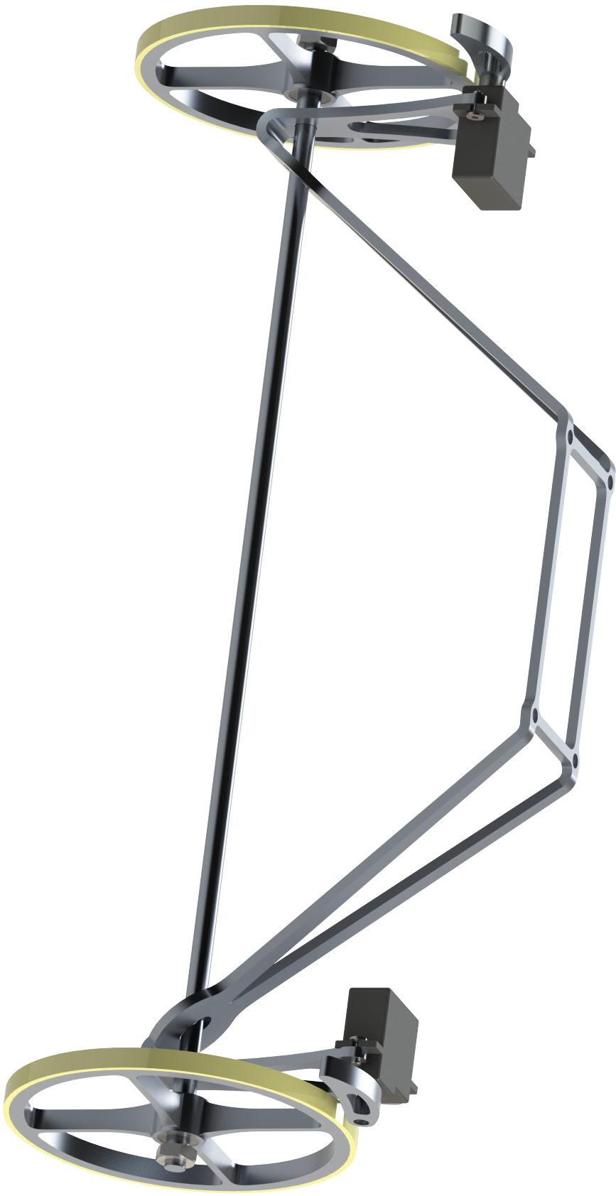
Figure 1 : Render of proposed redesign of UMSAE Aero team main landing gear
