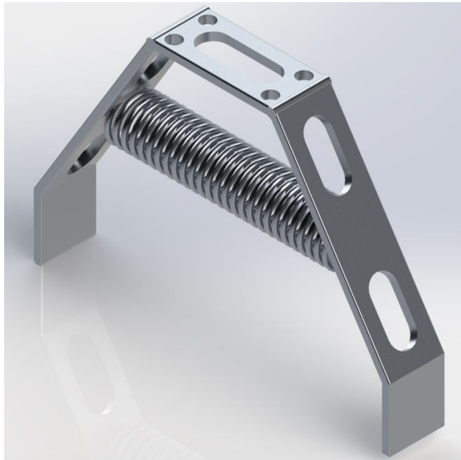
Figure 11: Main Landing Gear Concept 2 | Horizontal Spring with Hinge
