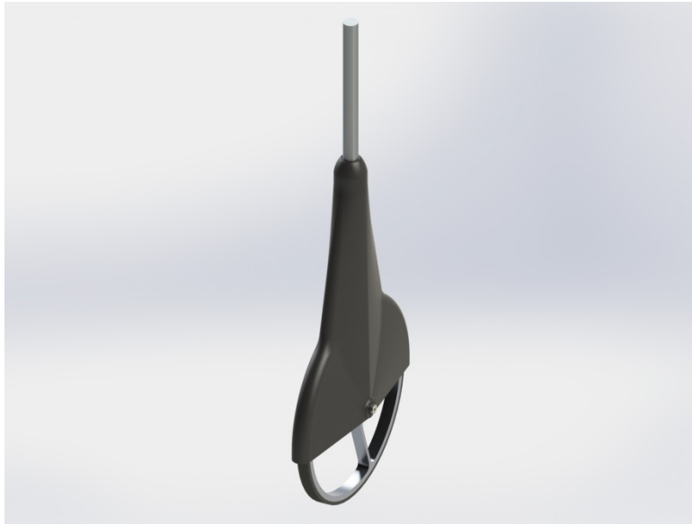
Figure 78: 3D printed solid link nose gear concept
