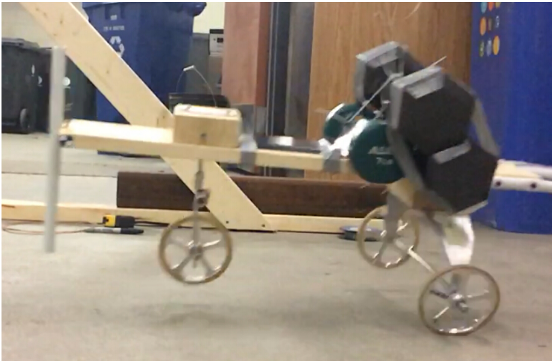
Figure 41: High speed footage frame at the point of contact of the main landing gear [29]
