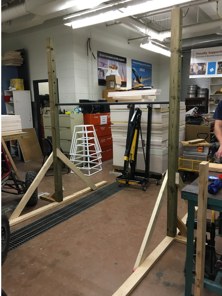
Figure 33: Swing drop test frame [24]
