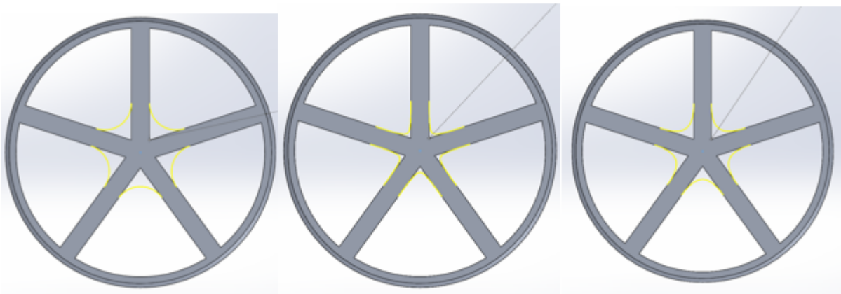
Figure 50: Circular, conic rho, and conic radius fillets for wheel redesign (from Left to Right)
