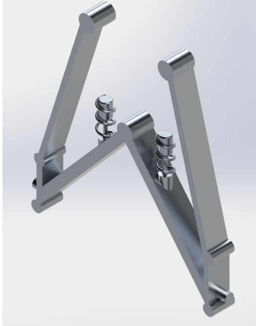
Figure 13: Main Landing Gear Concept 4 | Multilinked with Dampers
