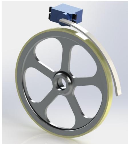
Figure 7: Braking System Concept 1 | Lever Style Braking System
