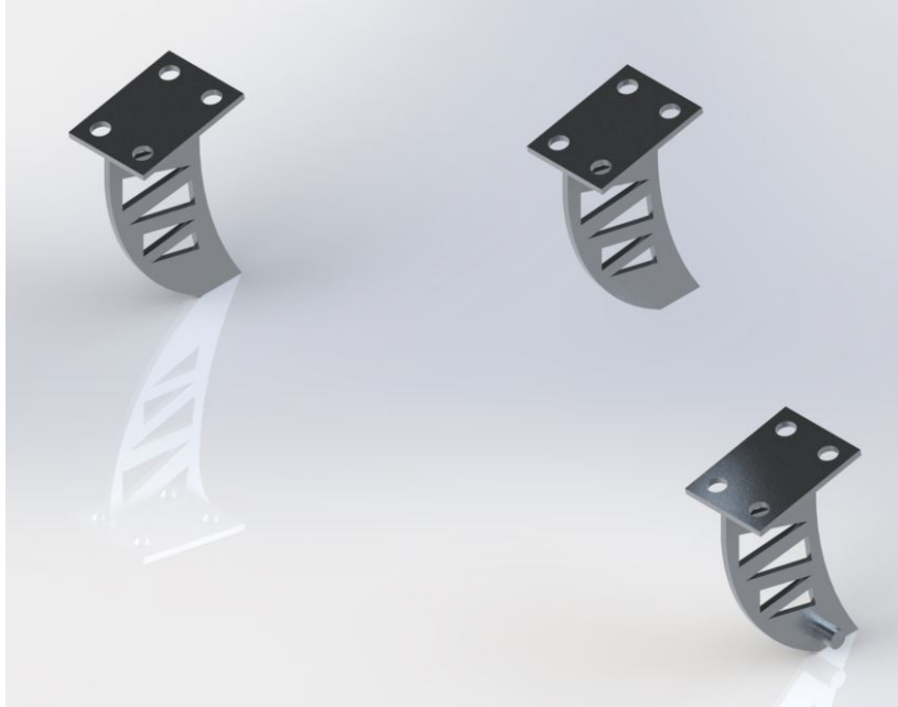
Figure 15: Main Landing Gear Concept 6 | Bicycle Style
