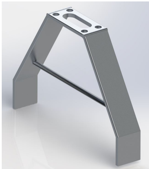
Figure 16: Main Landing Gear Concept 7 | Leaf Spring with Cable Concept
