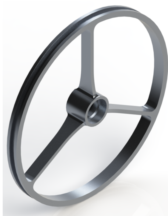
Figure 75: Final Render of the Nose Gear Wheel
