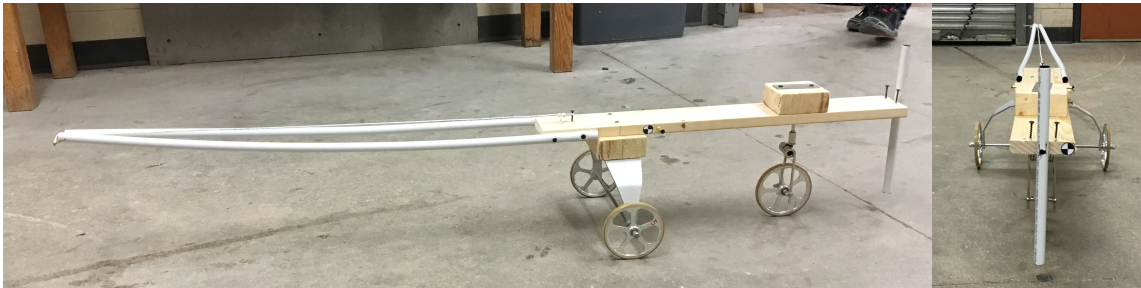
Figure 27: 2015 UMSAE Aero landing gear test chassis side view (left) and front view (right) [20]
