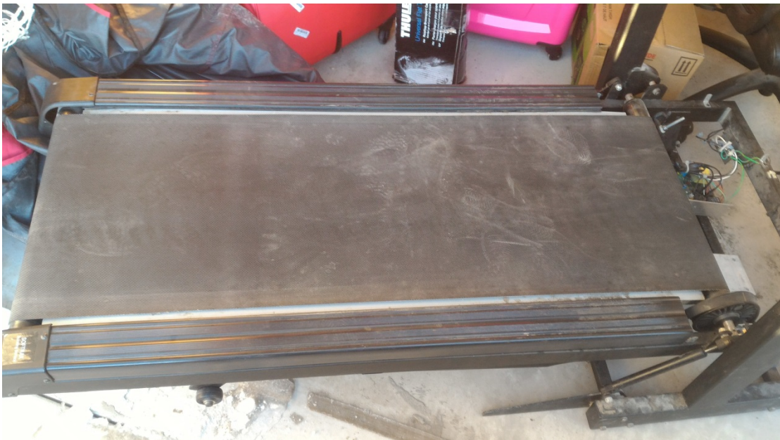
Figure 20: Treadmill acquired from Kijiji for permanent rolling resistance test rig
