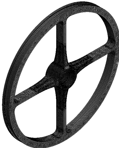
Figure 55: Sample of ANSYS mesh for FEA study
