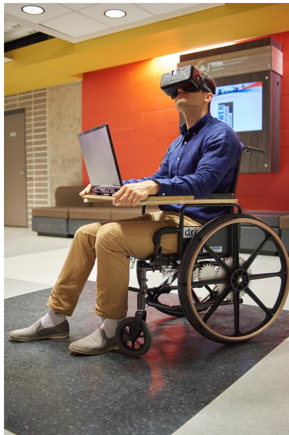
Fig. 3-21. VRNChair, based on an ordinary wheelchair.
