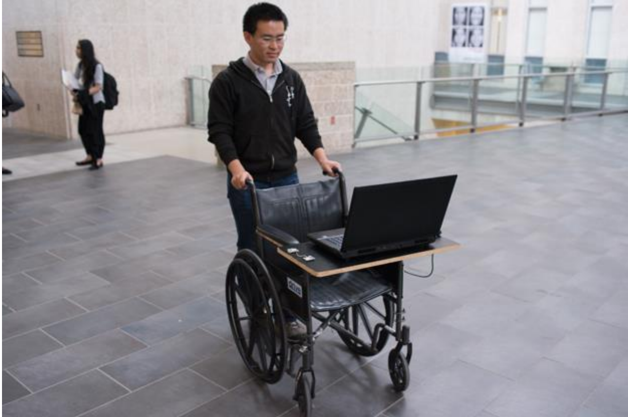
Fig. 4-6. VRNChair used with a laptop screen to interact with the virtual reality platform.
