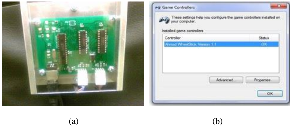
Fig. 3-24. VRNChair controller motion capture (a), Microsoft® Game Controller for VRNChair (b).
