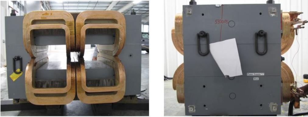
Fig. 6. Photos of the assembled septum yoke and coils. Front (left image) and side (right image) view of the septum magnet return yoke and coils. Centre shield is not shown.
