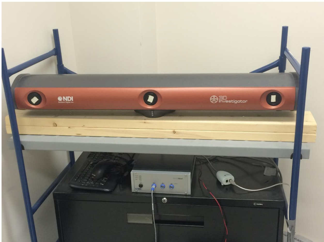
Figure 3. Optotrak 3D motion analysis system (Northern Digital, Inc.)
