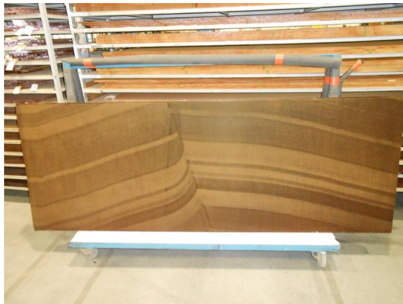
Figure 7: Core sheet experiencing partial cleaning (waviness) due to nozzle configuration.
