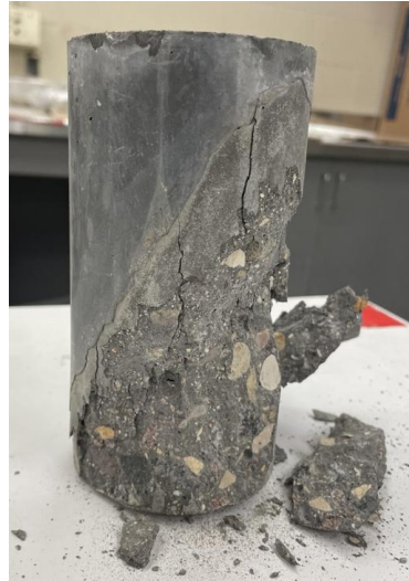
Figure 0.5: slant shear HSC Modes of failure
