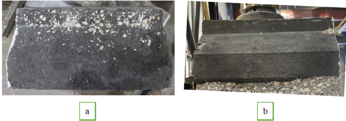
Figure 0.10: Failure surfaces of the (a) rough R-NR specimens, and (b) smooth S-NR
