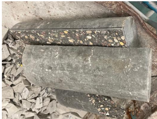
Figure 0.3: Indirect tension tests complete diametral splitting failure
