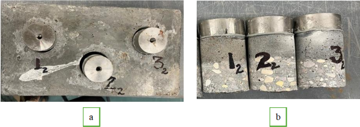
Figure 0.4: pull off test (a) pull off test specimen; (b) HSC failure
