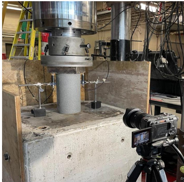
Figure 3.2: HSC specimen under compressive test
