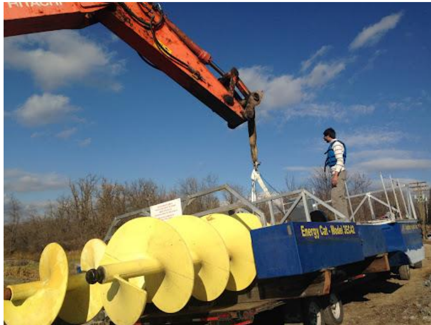
Figure 7: The deployment of an Archimedean RHKT at the CHTTC. The turbine features two counter-rotating screws, which can be inclined relative to the water flow to enhance overall water-to-wire efficiency. This innovative design aims to optimize energy capture from river currents, making it a promising solution for sustainable energy generation in riverine environments.
