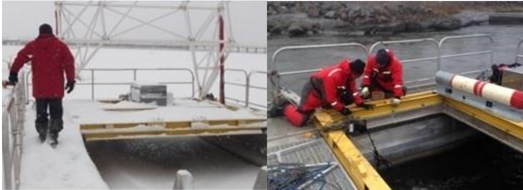
Figure 12: Challenges of a winter operation that inhibits regular procedures at the CHTTC: (left) floating support structure for the horizontal axis turbine is covered with snow, representing the ice accumulation on the pontoon, and (proper) survival suits are required for winter testing. If someone falls into the water, the suits will help to delay the onset of hypothermia but can do little if pushed below the ice cover.
