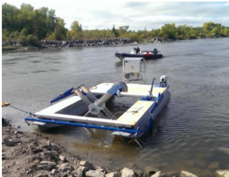
Figure 8: A 5-kW vertical-axis turbine developed by New Energy Corporation mounted on a specialized floating support structure at the CHTTC. The structure is designed for easy transportation to the desired location, where it can be anchored securely to a shore anchor or a granite block on the riverbed. This setup allows for efficient energy capture from river currents, contributing to the advancement of hydrokinetic energy technologies.
