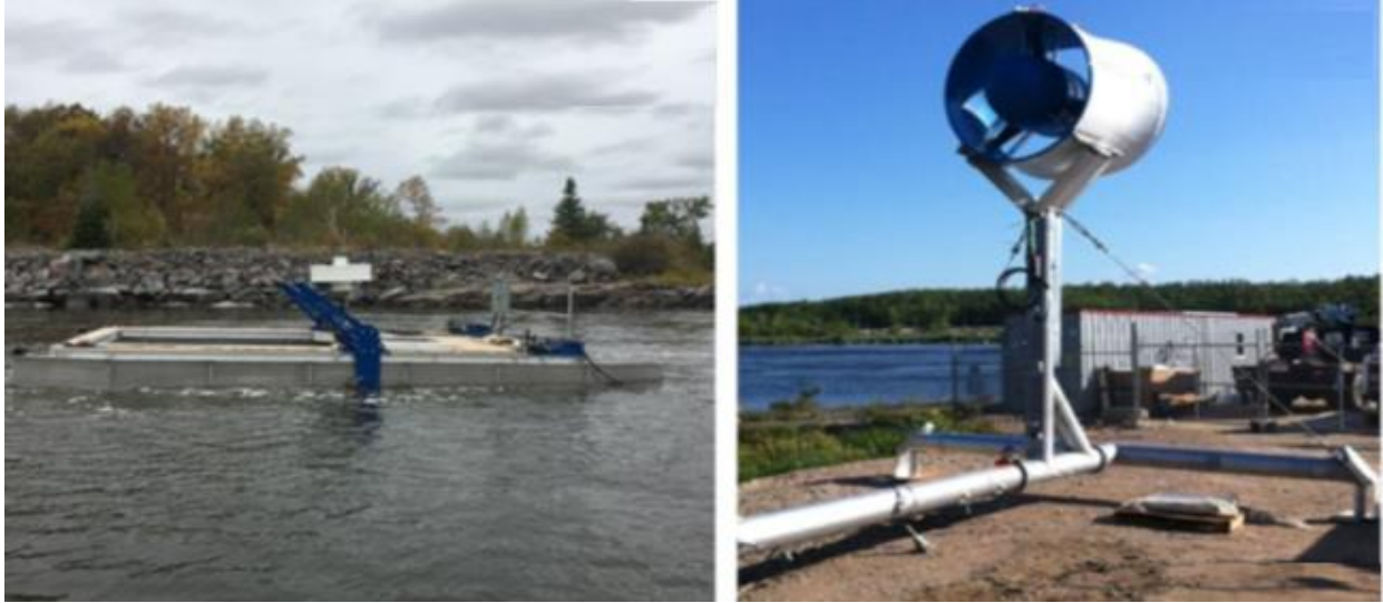
Figure 1: The Canadian Hydrokinetic Turbine Test Centre (CHTTC) evaluates different types of RHKT. The left image shows a near-surface RHKT positioned to maximize exposure to the free stream velocity. The right image depicts a bottom-mounted RHKT featuring a mounting structure that elevates the rotor above the boundary layer for optimal performance.
