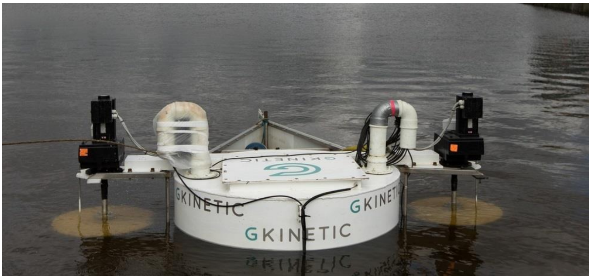
Figure 9: GKINetic's innovative vertical RHKT concept features two vertical rotors connected to micro-generators on either side. This design is engineered to harness the kinetic energy from flowing river water efficiently, enhancing power generation capabilities. The unique configuration of the vertical rotors allows for optimized energy capture, even in slow-moving water, making it a versatile solution for various riverine environments.
