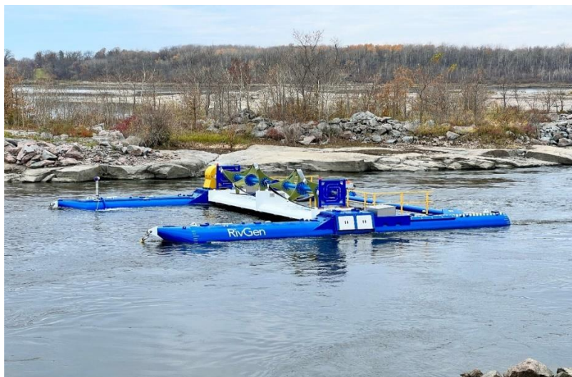
Figure 10: Before its submersion, the ORPC RivGen RHKT is being launched at the CHTTC on the Winnipeg River. The RivGen system is designed to generate renewable energy from river currents, providing a sustainable power solution for remote and off-grid communities. The deployment at CHTTC allows for comprehensive testing and evaluation of its performance and efficiency in real-world conditions.
