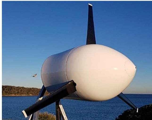
Figure 6: A Mako axial flow turbine with a 2 m diameter featuring a horizontal river turbine design equipped with three rotor blades. The turbine's relatively large rotor hub is engineered to accommodate a low-speed generator, eliminating the need for a gearbox. This design suits various applications, including tidal flows, rivers, irrigation canals, and tailraces.
