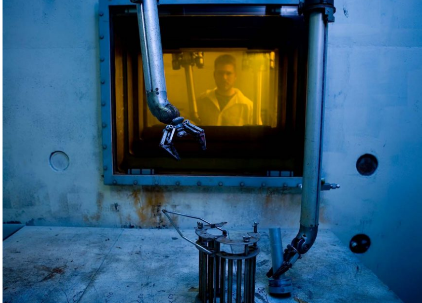
FIGURE 2.6: Picture of the Cobalt-60 test chamber at McMaster University [62].
