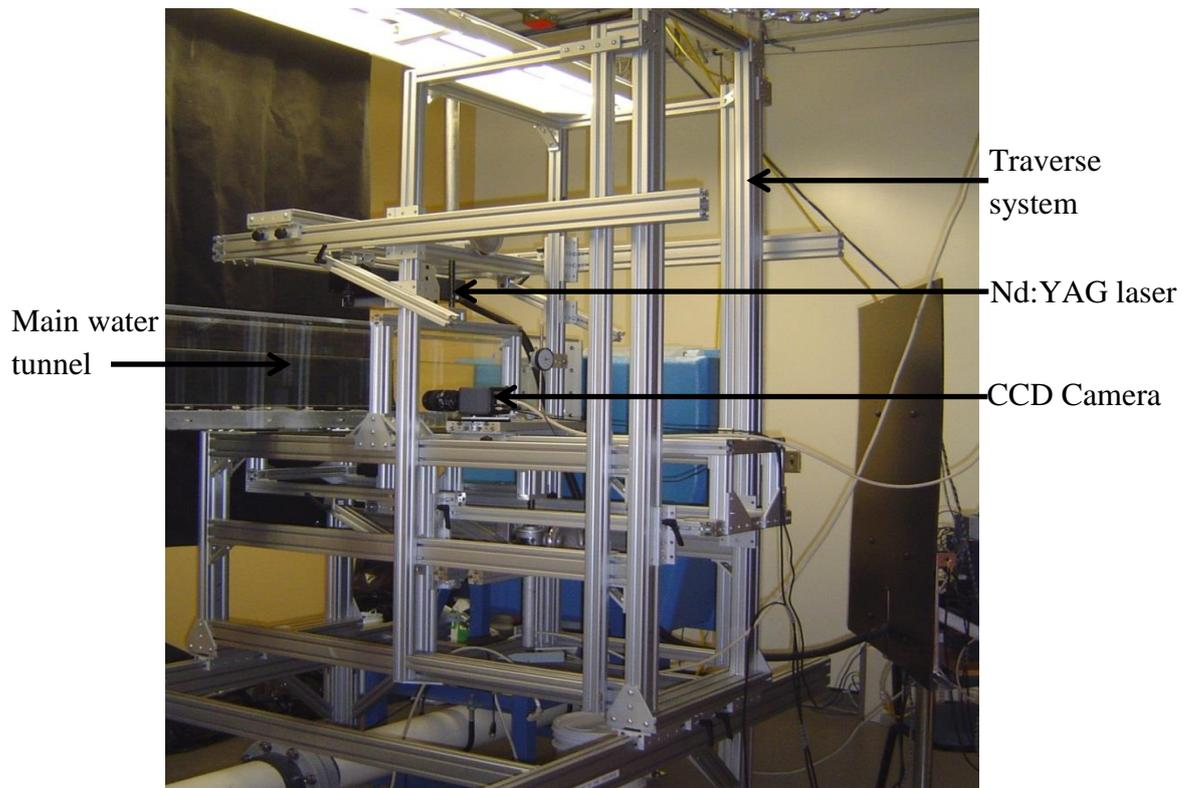
Figure 3.1: Experimental setup in the laboratory
