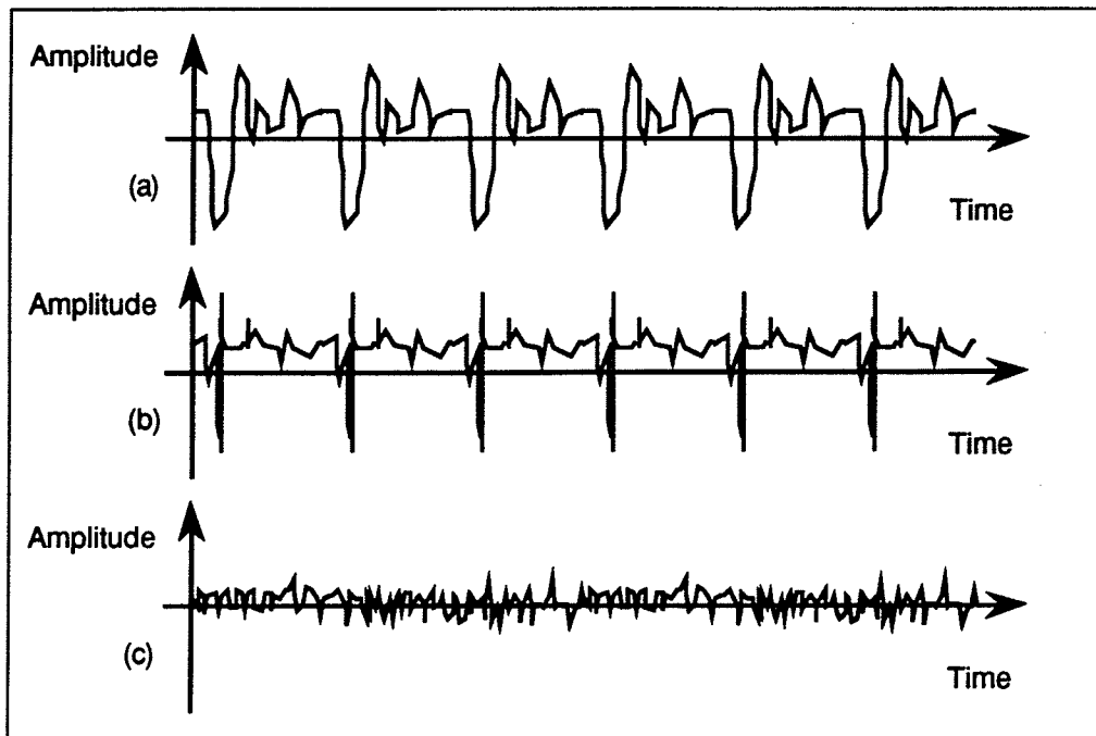
Fig. 2.15. Waveforms of different signals. (a) Original speech. (b) Original speech after an LP inverse filter, representing the excitation impulses. (c) Residual impulses as a result of applying the original speech to a cascade of the inverses of LP and pitch filters. The amplitudes of (b) and (c) are magnified by approximately 5 and 2 relative to (a), respectively. (After [ScAt85]).
