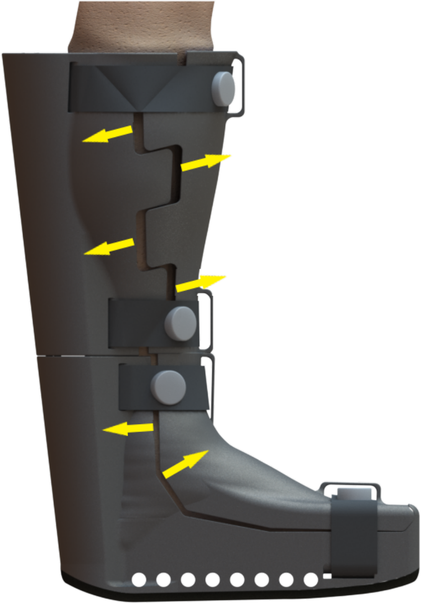
Figure 20: CROW Boot with Expansion Shown by Yellow Arrows
