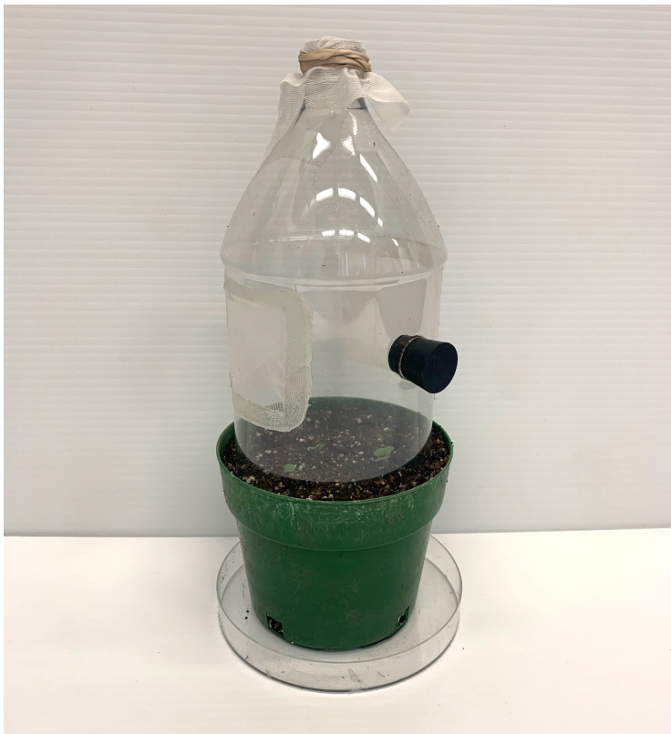
Figure 2.2. Microcosm set up consisting of circular plastic pot (950.5 cm 3 ) and a plastic covering made from the top portion of a 2L plastic pop bottle (23 cm height x 11 cm diameter).
