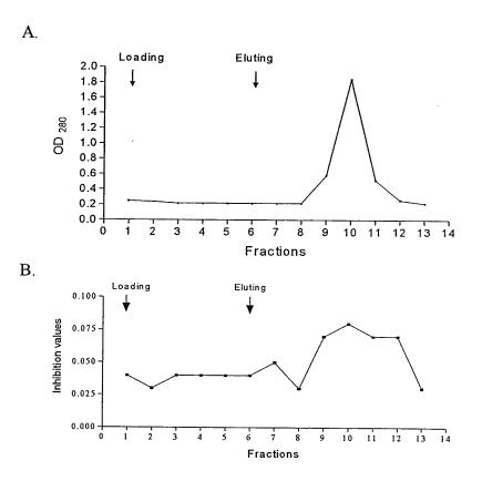
Figure 18 A. Purification of rAFXa using DEAE–Sephacel chromatography The concentrated rAFXa supernatant was dialyzed against Tris buffer (20 mM pH 8.0), centrifuged and then loaded onto a DEAE-Sephacel column equilibrated with the same buffer. After washing the column with the same buffer, the bound proteins were eluted with a linear gradient of NaCl from 0 to 1 M in the Tris buffer. Fractions were collected and monitored for protein concentration using a Biological Data view machine (OD 280).
