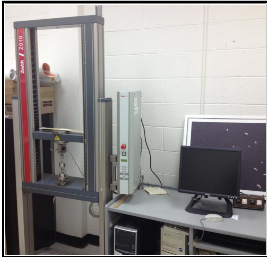
Figure 5.2.3.2: Zwick Universal testing machine and computer
