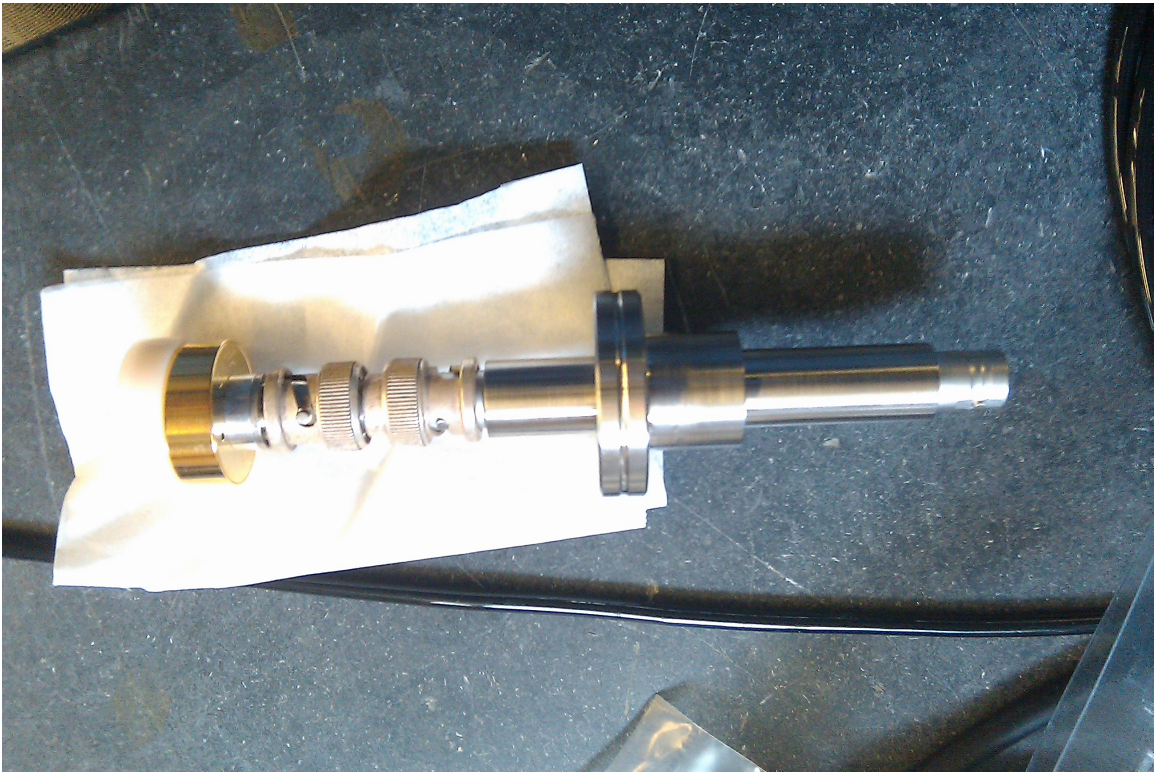
Figure 3.8: Ortec model CU-012-100-300 silicon detector mounted on a 1.33" CF BNC feedthrough.
