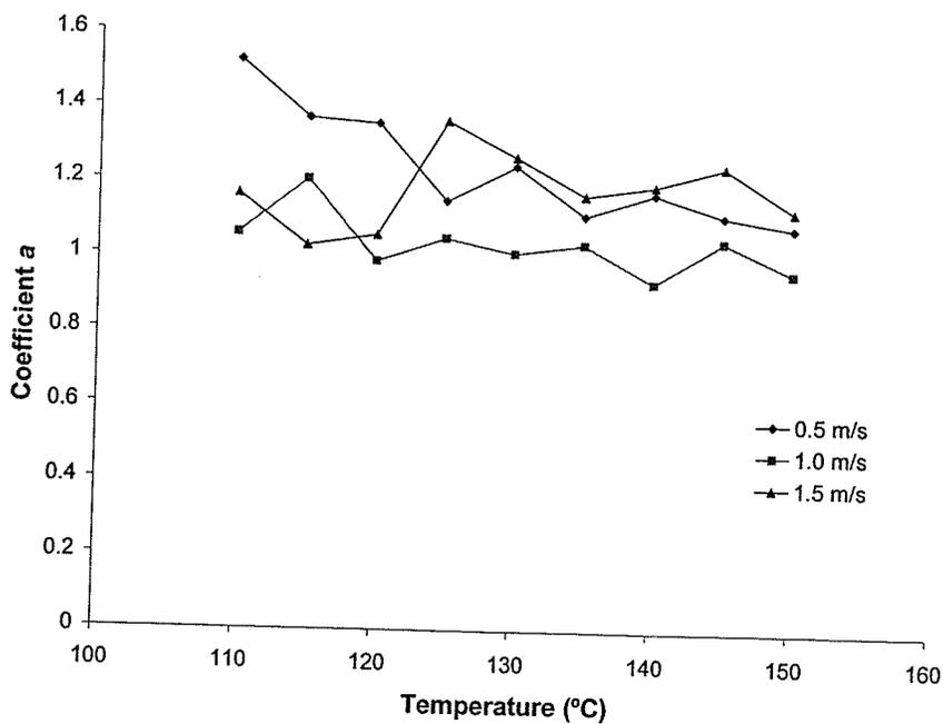
(b) Changes in coefficient  $a$  with steam temperature
