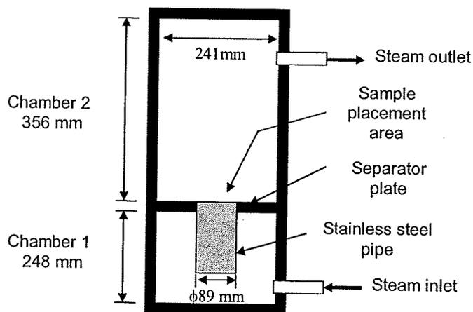
Fig. 3.2. Drying chamber of superheated steam drying system.
