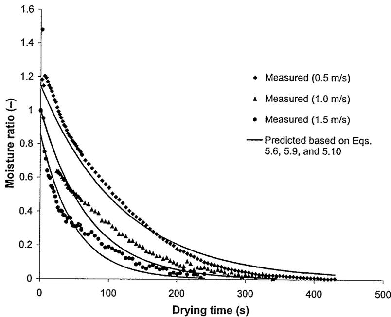
Fig. 5.8. Comparison of predicted results and measured values of moisture ratio for noodles processed in superheated steam at 140°C and velocities of 0.5, 1.0, and 1.5 m/s.
