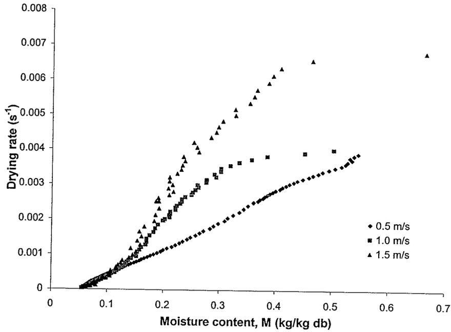
Fig. 5.16. Predicted drying rates for noodles processed in superheated steam at 135°C and velocities of 0.5, 1.0, and 1.5 m/s.
