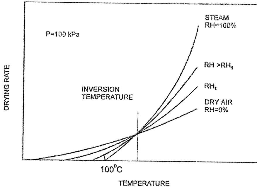
Fig. 2.1. Drying rate vs. temperature for air and steam (Kudra and Mujumdar 2002).
