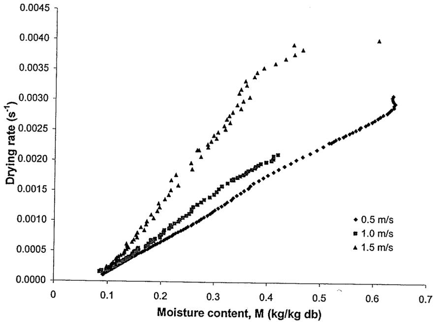
Fig. 5.13. Predicted drying rates for noodles processed in superheated steam at 120°C and velocities of 0.5, 1.0, and 1.5 m/s.
