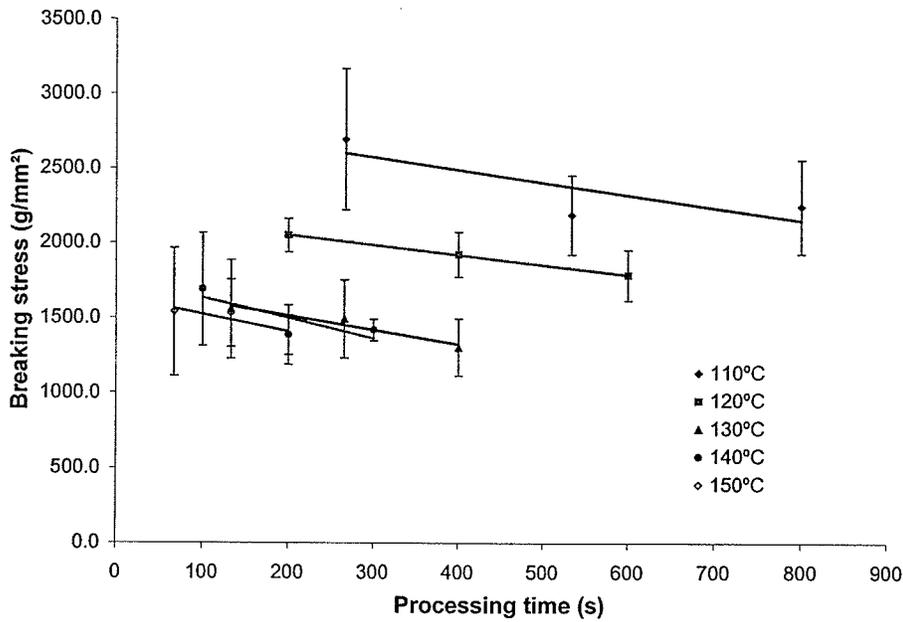
Fig. 5.29. Breaking stress of noodles processed in superheated steam at a velocity of 1.0 m/s and temperatures of 110, 120, 130, 140, and 150°C.
