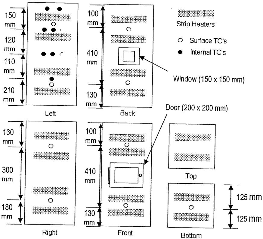
Fig. 3.3. Diagram of strip heater and thermocouple (TC) placement on exterior of the drying chamber (Gervais et al. 2004).
