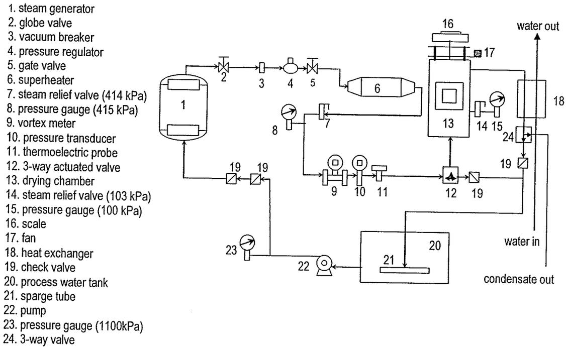
Fig. 3.1. Schematic of the superheated steam processing system.
