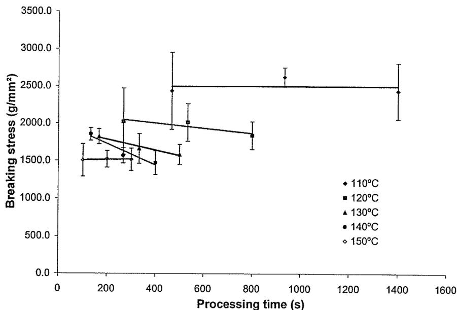
Fig. 5.28. Breaking stress of noodles processed in superheated steam at a velocity of 0.5 m/s and temperatures of 110, 120, 130, 140, and 150°C.
