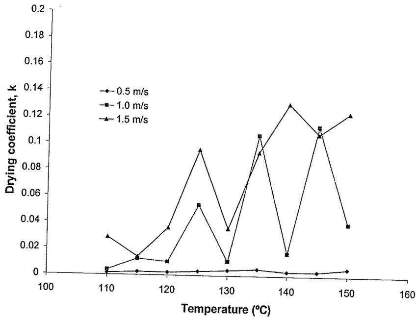
(b) Changes in drying coefficient  $k$  with steam temperature
