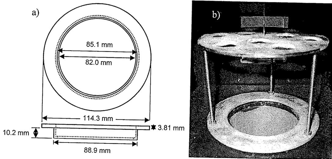
Fig. 4.4. Sample tray (a) and holder (b) used for mass measurement during superheated steam drying.
