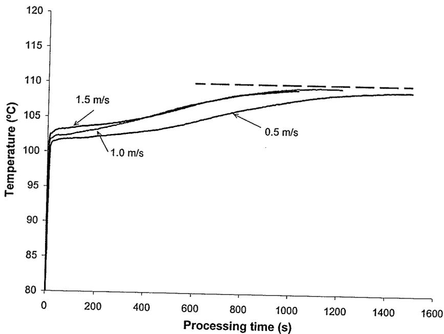
Fig. 5.20. Internal temperature measured near the geometric centre for noodles processed in superheated steam at 110°C and velocities of 0.5, 1.0, and 1.5 m/s (--- medium temperature).
