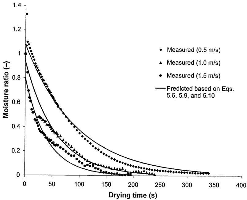
Fig. 5.10. Comparison of predicted results and measured values of moisture ratio for noodles processed in superheated steam at 150°C and velocities of 0.5, 1.0, and 1.5 m/s.
