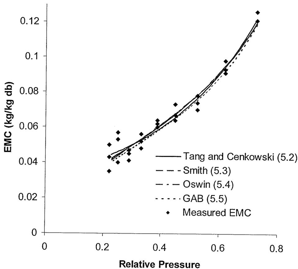
Fig. 5.1. Predicted and measured EMC of Asian noodles processed in superheated steam at 104.7kPa
