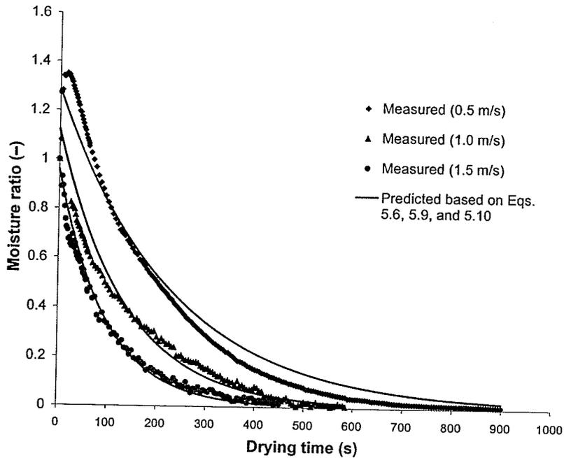
Fig. 5.4. Comparison of predicted results and measured values of moisture ratio for noodles processed in superheated steam at 120°C and velocities of 0.5, 1.0, and 1.5 m/s.
