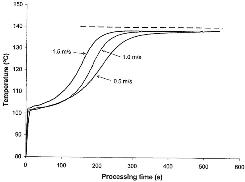
Fig. 5.23. Internal temperature measured near the geometric centre for noodles processed in superheated steam at 140°C and velocities of 0.5, 1.0, and 1.5 m/s (— — — medium temperature).
