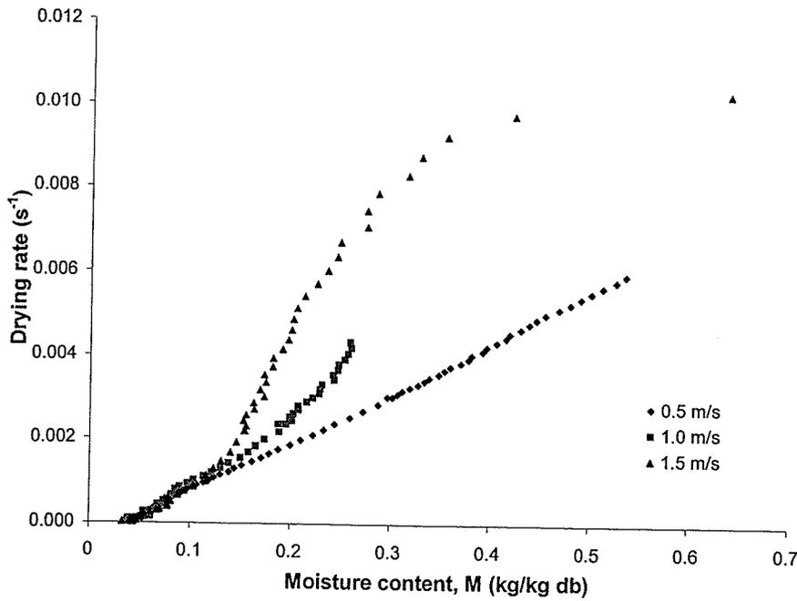
Fig. 5.19. Predicted drying rates for noodles processed in superheated steam at 150°C and velocities of 0.5, 1.0, and 1.5 m/s.
