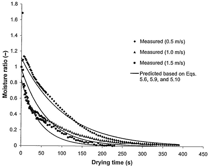
Fig. 5.9. Comparison of predicted results and measured values of moisture ratio for noodles processed in superheated steam at 145°C and velocities of 0.5, 1.0, and 1.5 m/s.
