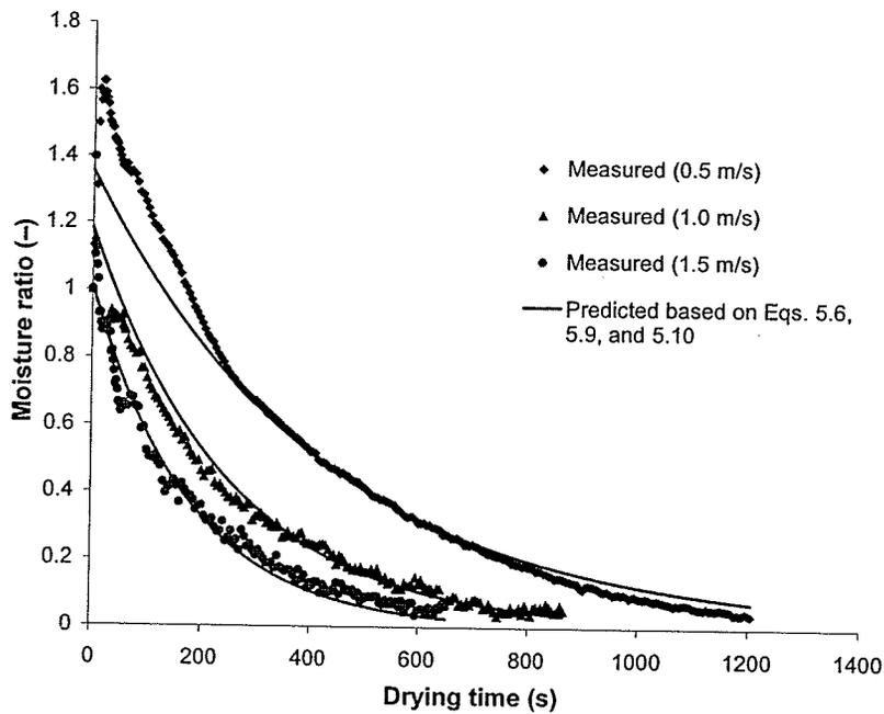
Fig. 5.2. Comparison of predicted results and measured values of moisture ratio for noodles processed in superheated steam at 110°C and velocities of 0.5, 1.0, and 1.5 m/s.
