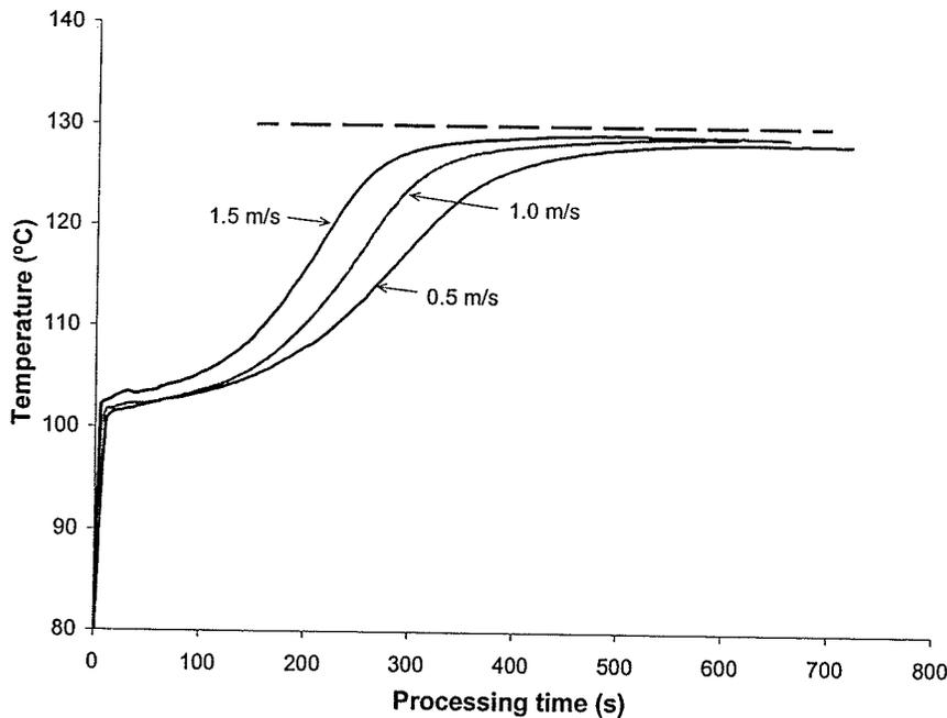
Fig. 5.22. Internal temperature measured near the geometric centre for noodles processed in superheated steam at 130°C and velocities of 0.5, 1.0, and 1.5 m/s (--- medium temperature).
