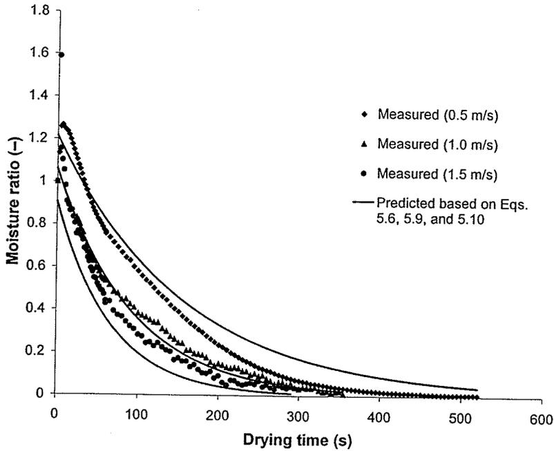
Fig. 5.6. Comparison of predicted results and measured values of moisture ratio for noodles processed in superheated steam at 130°C and velocities of 0.5, 1.0, and 1.5 m/s.
