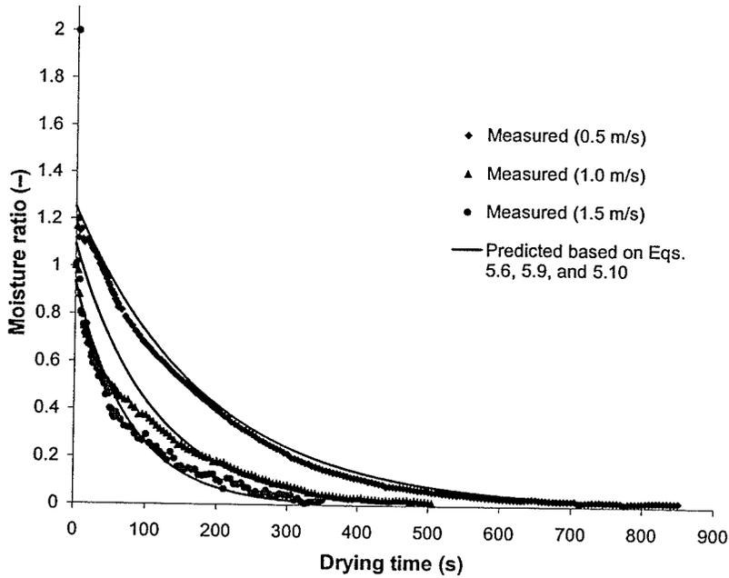
Fig. 5.5. Comparison of predicted results and measured values of moisture ratio for noodles processed in superheated steam at 125°C and velocities of 0.5, 1.0, and 1.5 m/s.
