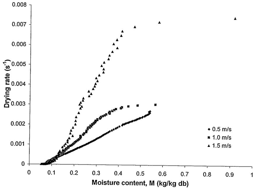
Fig. 5.14. Predicted drying rates for noodles processed in superheated steam at 125°C and velocities of 0.5, 1.0, and 1.5 m/s.
