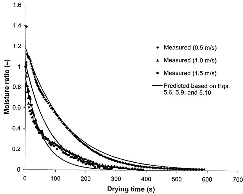
Fig. 5.7. Comparison of predicted results and measured values of moisture ratio for noodles processed in superheated steam at 135°C and velocities of 0.5, 1.0, and 1.5 m/s.
