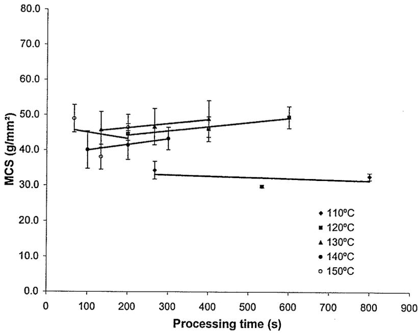
Fig. 5.26. Maximum cutting stress of noodles processed in superheated steam at a velocity of 1.0 m/s and temperatures of 110, 120, 130, 140, and 150°C.
