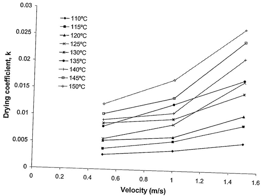
(a) Changes in drying coefficient  $k$  with steam velocity
