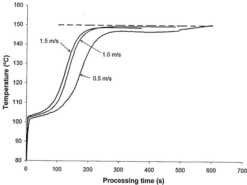
Fig. 5.24. Internal temperature measured near the geometric centre for noodles processed in superheated steam at 150°C and velocities of 0.5, 1.0, and 1.5 m/s (— — — medium temperature).
