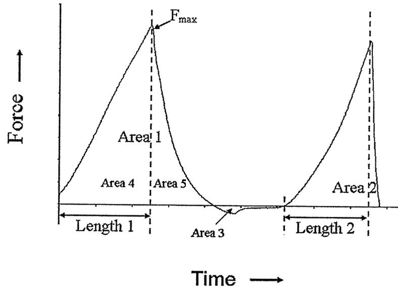
Fig. 2.7. Typical TPA curve for alkaline noodles using the TA-XT2i showing measurements used to calculate textural properties.
