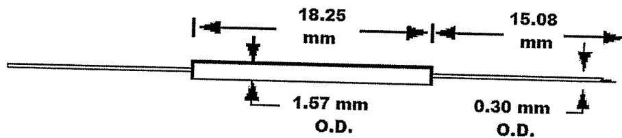
Fig. 4.5. Needle probe dimensions.
