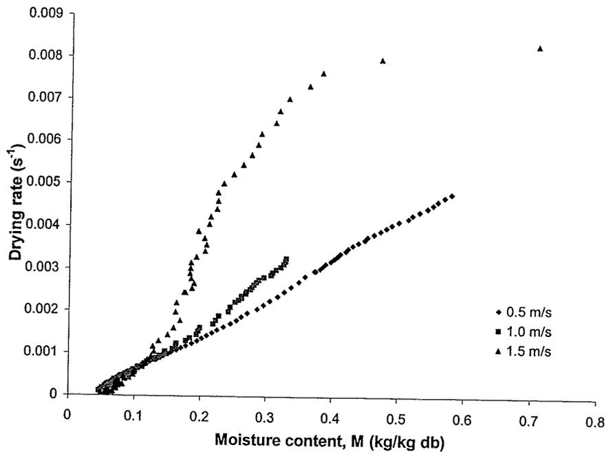
Fig. 5.17. Predicted drying rates for noodles processed in superheated steam at 140°C and velocities of 0.5, 1.0, and 1.5 m/s.
