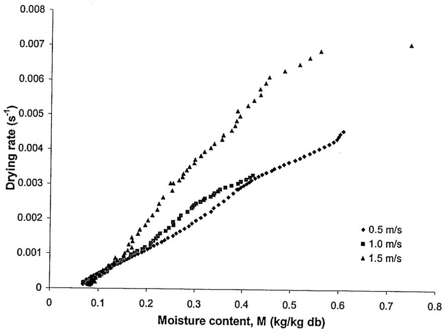
Fig. 5.15. Predicted drying rates for noodles processed in superheated steam at 130°C and velocities of 0.5, 1.0, and 1.5 m/s.
