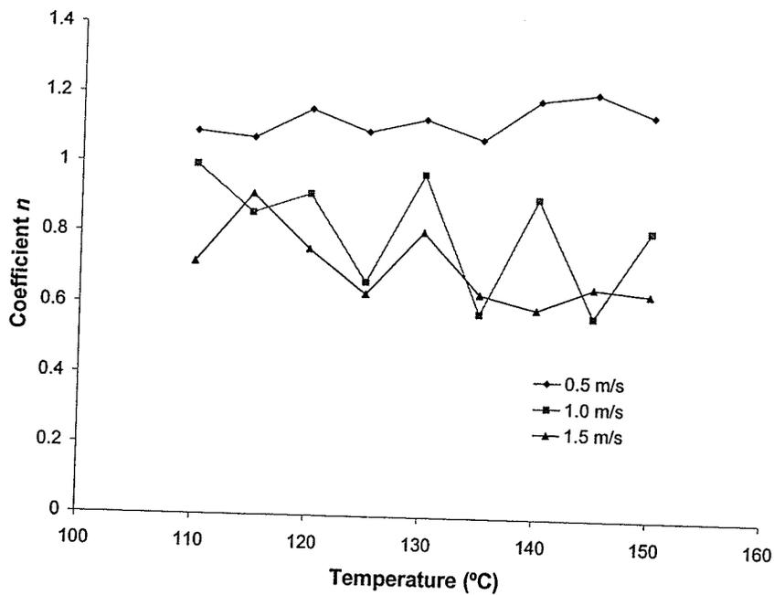
(b) Changes in coefficient  $n$  with steam temperature
