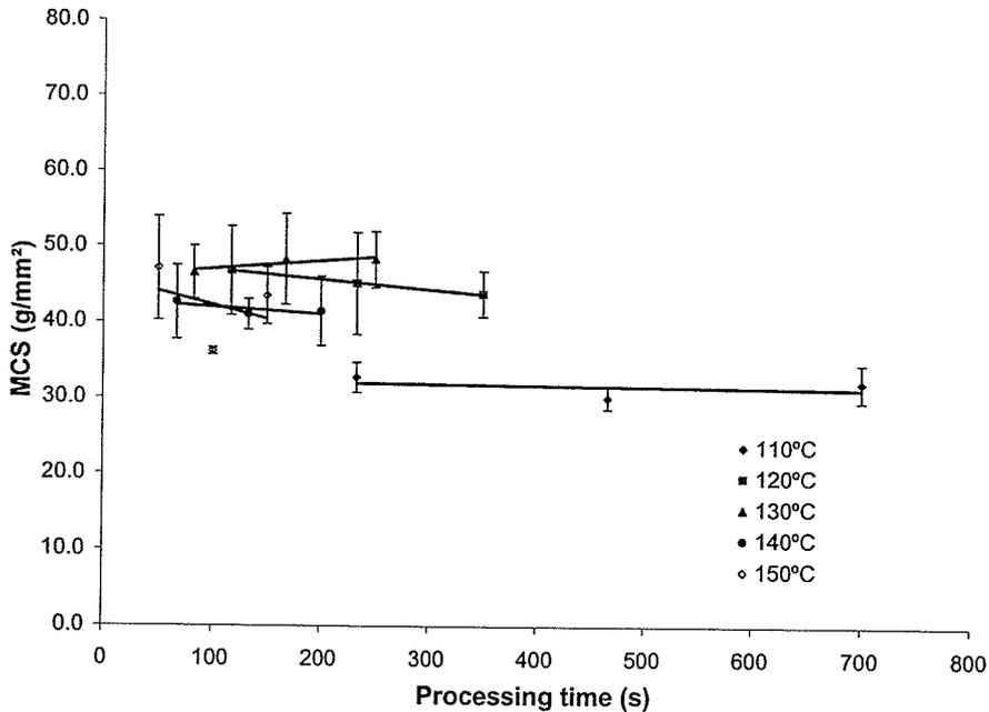
Fig. 5.27. Maximum cutting stress of noodles processed in superheated steam at a velocity of 1.5 m/s and temperatures of 110, 120, 130, 140, and 150°C.
