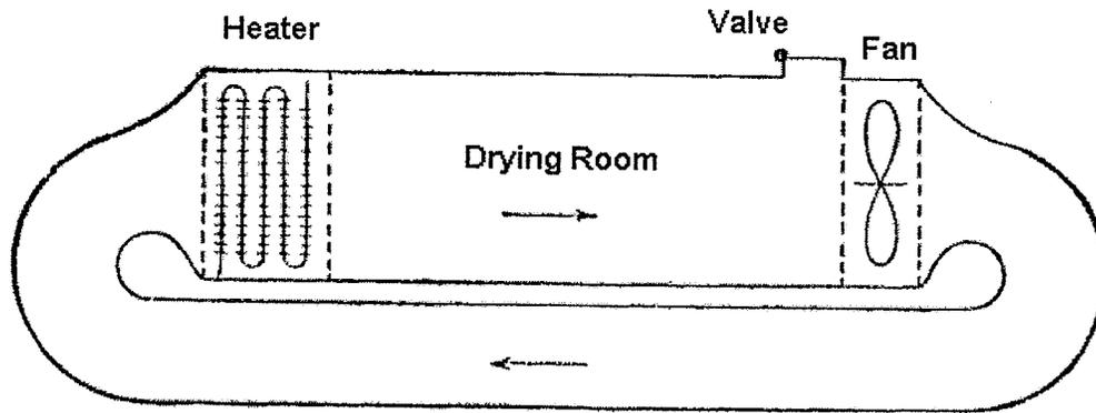
Fig. 2.2. Simple superheated steam dryer (modified from Hausbrand 1912).
