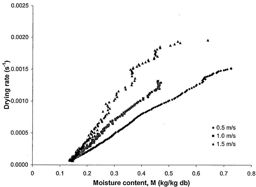
Fig. 5.11. Predicted drying rates for noodles processed in superheated steam at 110°C and velocities of 0.5, 1.0, and 1.5 m/s.
