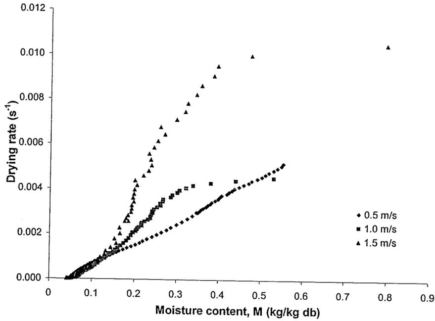
Fig. 5.18. Predicted drying rates for noodles processed in superheated steam at 145°C and velocities of 0.5, 1.0, and 1.5 m/s.
