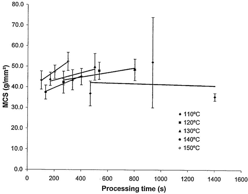
Fig. 5.25. Maximum cutting stress of noodles processed in superheated steam at a velocity of 0.5 m/s and temperatures of 110, 120, 130, 140, and 150°C.
