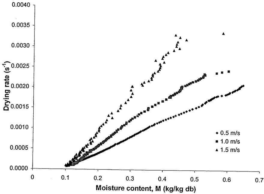
Fig. 5.12. Predicted drying rates for noodles processed in superheated steam at 115°C and velocities of 0.5, 1.0, and 1.5 m/s.
