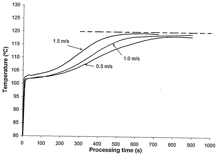
Fig. 5.21. Internal temperature measured near the geometric centre for noodles processed in superheated steam at 120°C and velocities of 0.5, 1.0, and 1.5 m/s (--- medium temperature).
