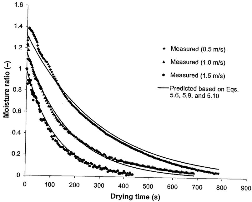
Fig. 5.3. Comparison of predicted results and measured values of moisture ratio for noodles processed in superheated steam at 115°C and velocities of 0.5, 1.0, and 1.5 m/s.
