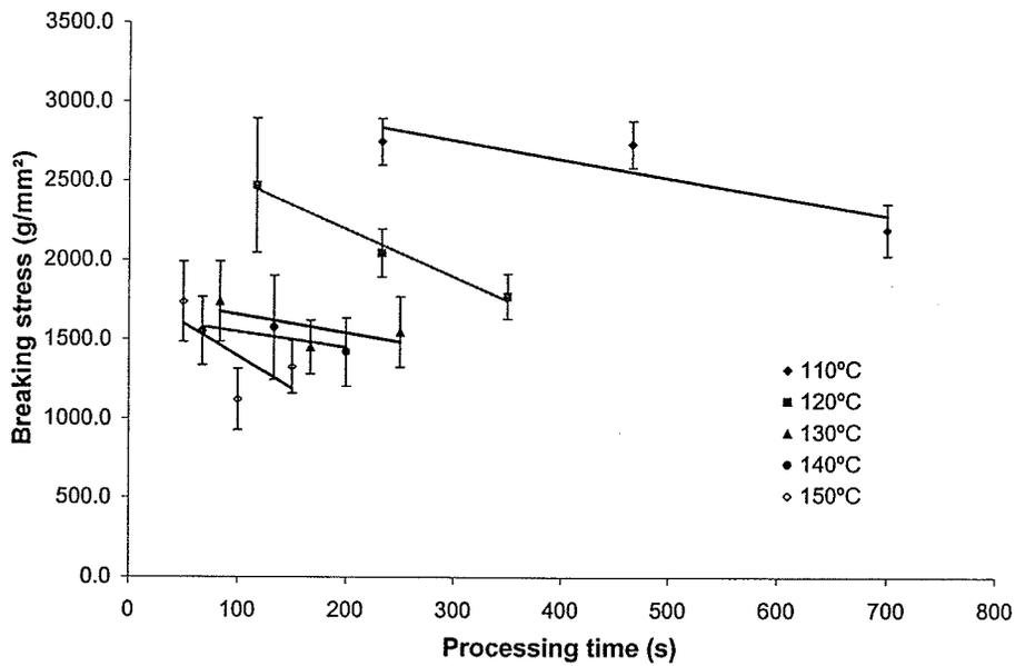
Fig. 5.30. Breaking stress of noodles processed in superheated steam at a velocity of 1.5m/s and temperatures of 110, 120, 130, 140, and 150°C.
