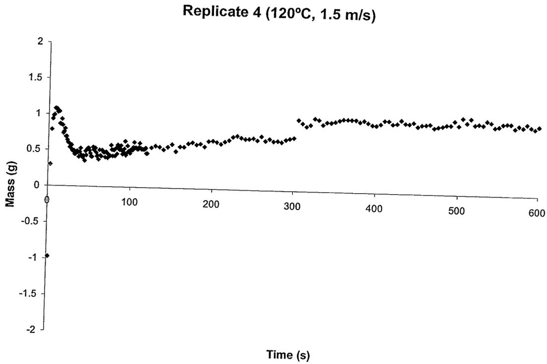
Fig. A1.1. Mass change experiment where noodle strands that were longer than 15 mm curled up resulting in a decrease in lifting force and an increased mass reading.
