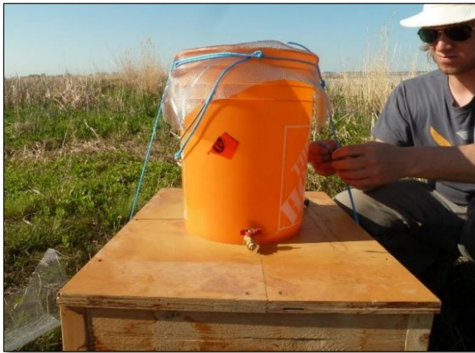
Figure 3.5 - Plastic bucket used for precipitation sample collection
