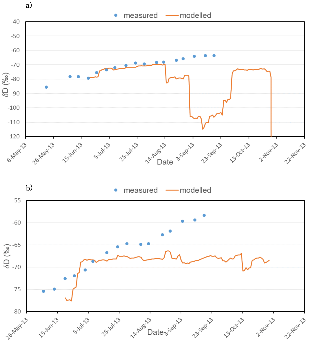
Figure A.7 – Fraction dependent model 2013; comparison of measured and modelled isotopic composition of \delta D – of a) western and b) eastern CFSTRs. Reference point for the western CFSTR is 25MC and 46MS for the eastern CFSTR.
