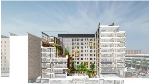
Fig 10. Carving away five storeys on the south side during the renovation, allows the courtyard to bring daylight deeper into the building. Source: VMDO Architects, 2022.
