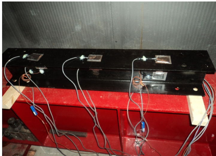
Fig.6. Steel test sample (with all sensors bonded)
