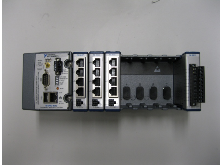
Fig. 7. NI cRIO-9012 (with NI 9237 and 9211 modules)
