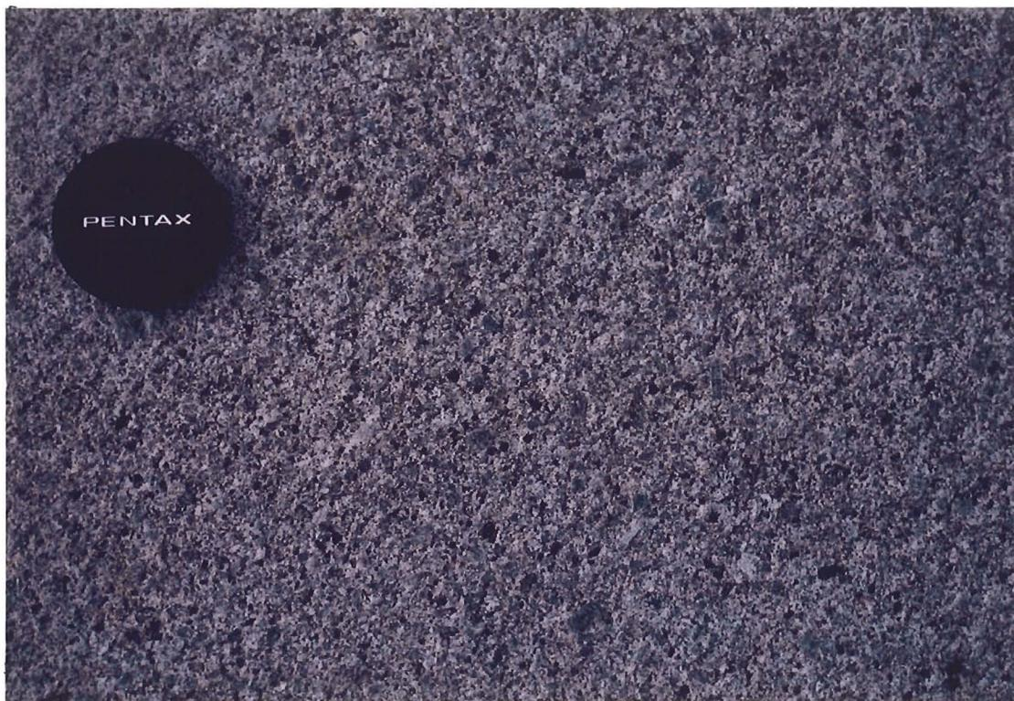
PLATE 14: Fine grained porphyritic quartz monzonite.
