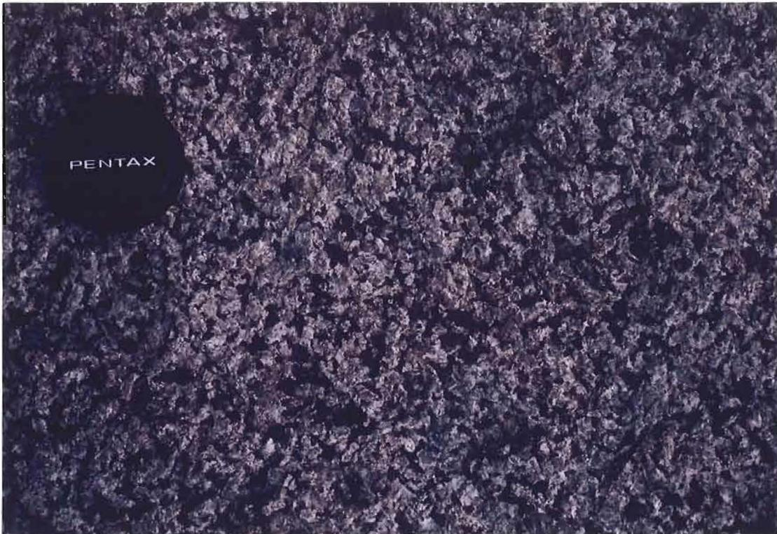
PLATE 5: Gabbro #3 displaying orthocumulus texture defined by a framework of coarse grained plagioclase crystals with irregular interstitial clots of mafic minerals.
