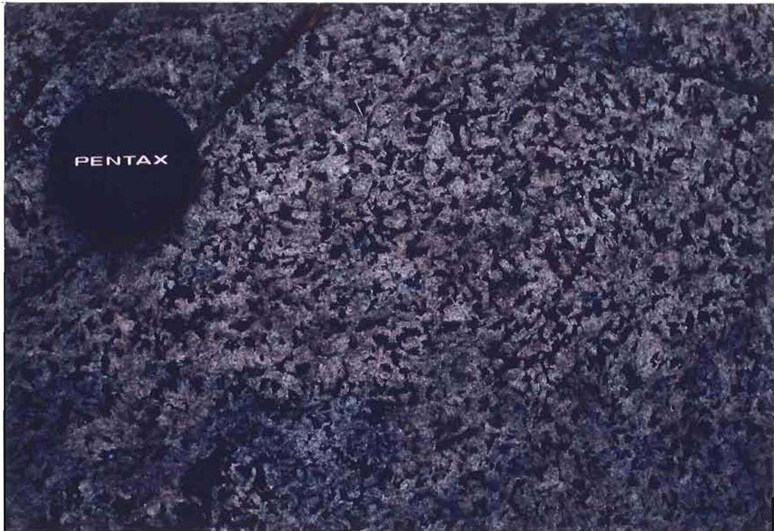
PLATE 9: Orthocumulate to mesocumulate Gabbro #4 comprised of coarse grained subhedral to euhedral lath-shaped plagioclase grains (white) and irregular intercumulus aggregates of mafic minerals (black).
