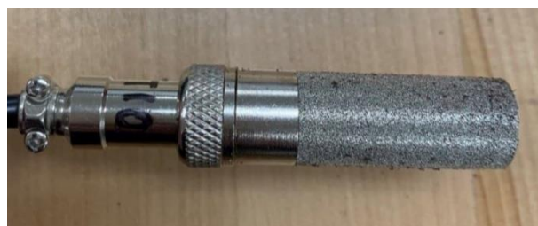
Figure 3.3. Soil temperature and moisture sensor.
