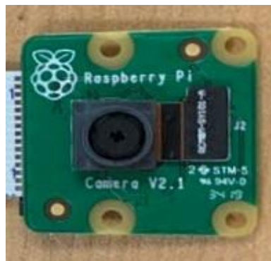
Figure 3.4. Raspberry Pi camera board V2 (8 MP).
