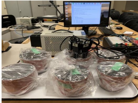
Figure 3.8 Calibration of soil temperature and moisture sensors for five moisture levels of soil.
