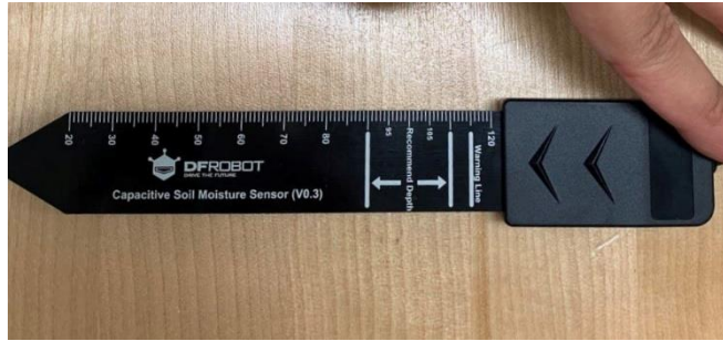
Figure 3.2. Analog waterproof capacitive soil moisture sensor.
