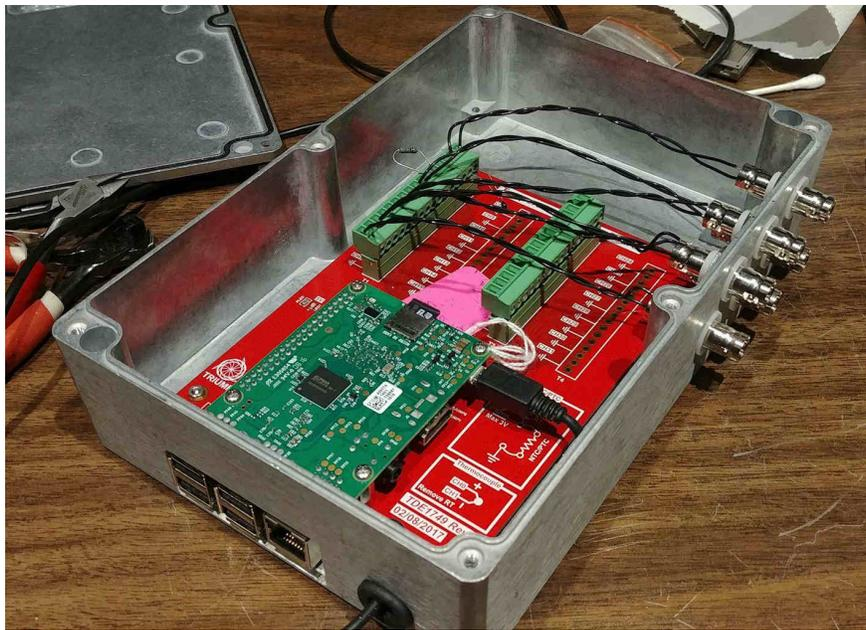
Figure 2.4: Raspberry Pi (R-Pi) computer for monitoring and logging ULE and room temperature data.
