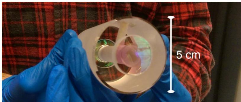
Figure 2.1: This is an image of our ULE cavity in hand.
