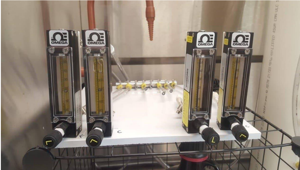
Figure B- 19. Flow meters to measure air injection inflow (Left) and the columns outflow (Right)
