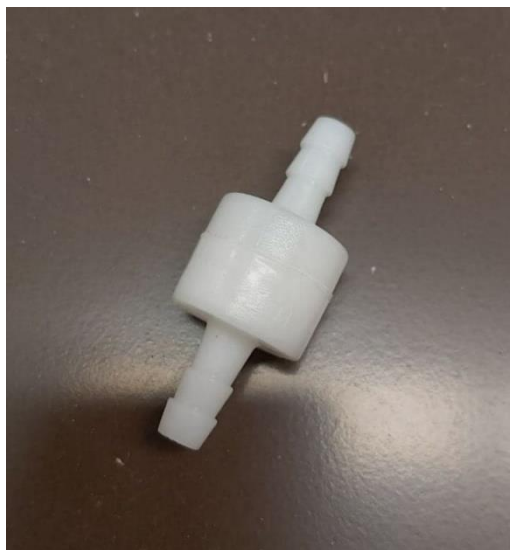
Figure B- 18. Check valve to make one-way synthetic LFG flow and prevent back flush to the gas tanks
