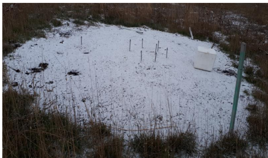
Figure A -8. The in situ bio-window with gas probes installed in winter
