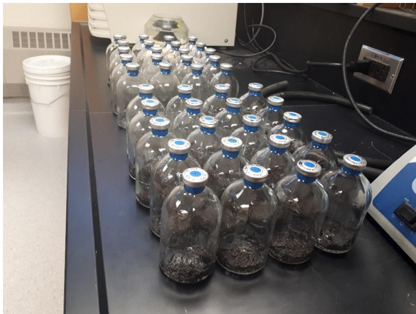
Figure A -9. Batch tests with 2 g of compost in 120 ml bottles
