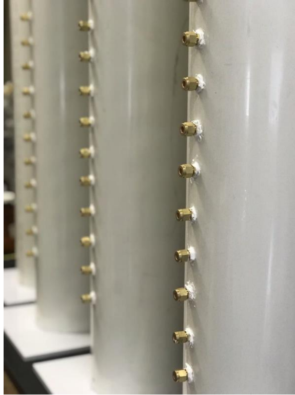
Figure B- 13. Installing the sampling ports equipped with gas tight septa
