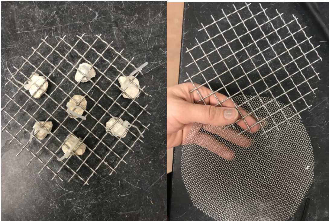
Figure B- 14. Coarse mesh with gravels attached for placement beneath the GDL to distribute the synthetic LFG homogeneously (Left). Fine mesh to place between layers of packing materials (GDL, Compost and gravel, compost) to prevent them mixing (Right, bottom)
