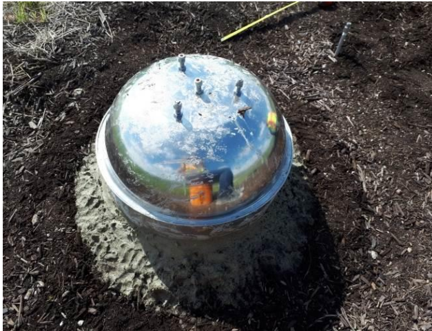
Figure A -4. Flux chamber sealed by bentonite and gas sampling for the flux measurement
