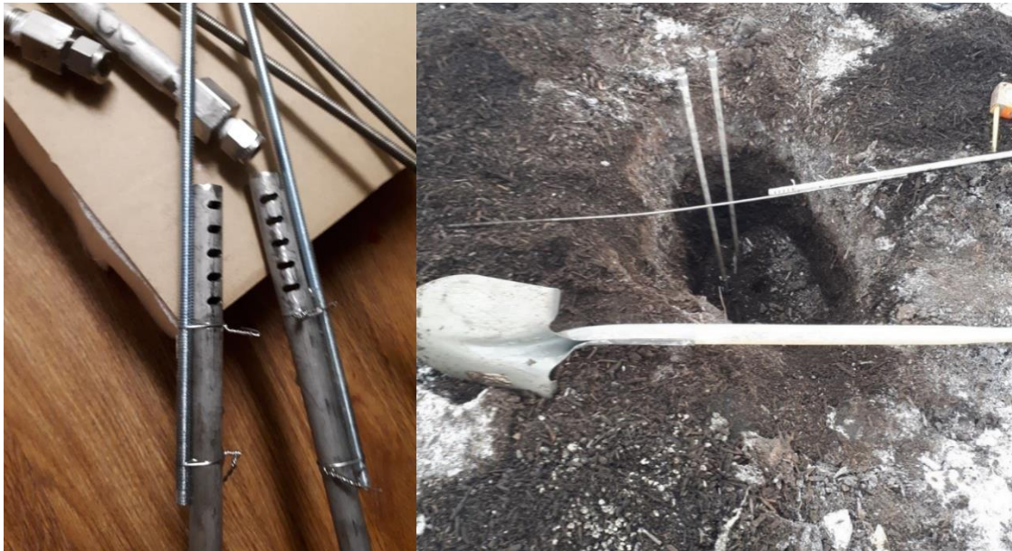
Figure A -2. Placement of probes with metal bars fixed in the GDL to make a deep foundation preventing the probe heave and displacement
