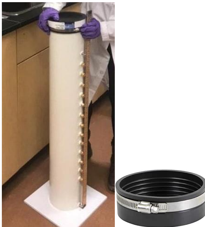
Figure B- 15. The packed column with PVC base plate and Flexible PVC Pipe Cap with Stainless Steel Clamps
