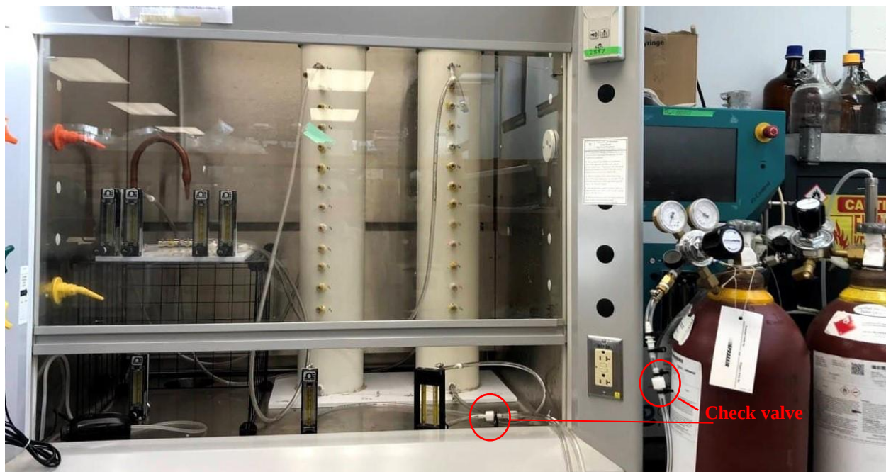
Figure B- 17. The final set-up of the column test with flow meters under the hood and gas tanks with pressure controlling valves and regulators
