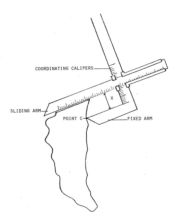
Figure 6: Method of Determining Measure X
