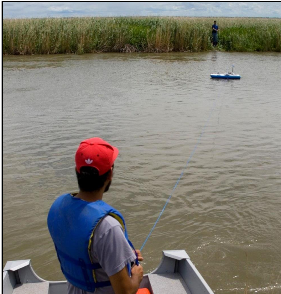
Figure 4:2 – Typical ADCP Operation
