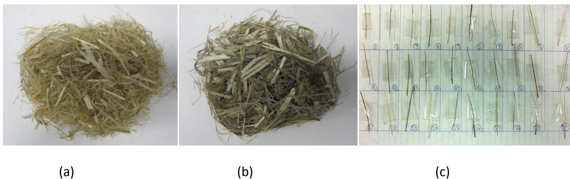
Fig. 4.3. Hemp materials; (a) processed unretted hemp, (b) processed retted hemp, (c) hemp fibre samples prepared for tensile tests.
