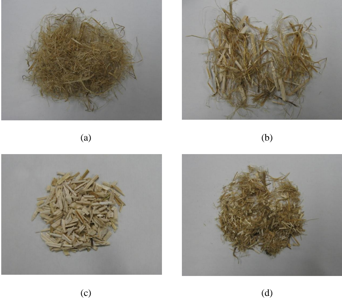
Fig. 6.3. Different fractions of the feedstock; (a) fibre, (b) fibre bound to core, (c) core, (d) chaff.
