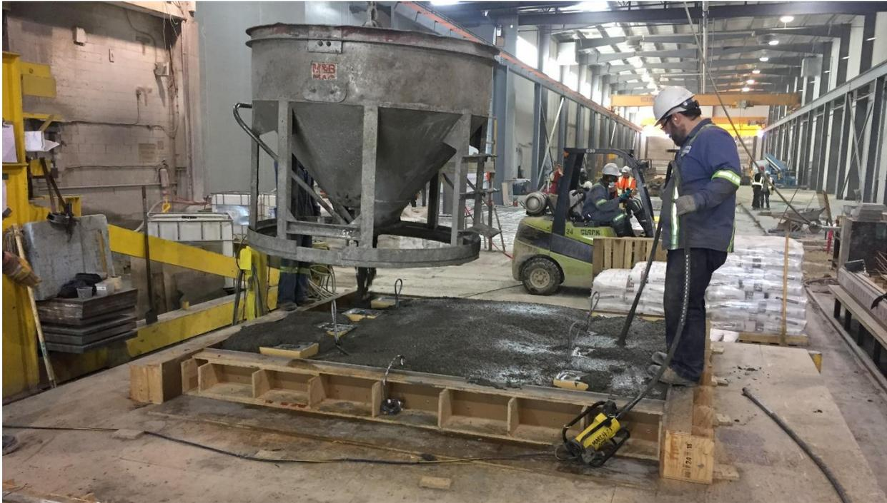
Figure 3.20 JPD half panel concrete casting and vibrating.
