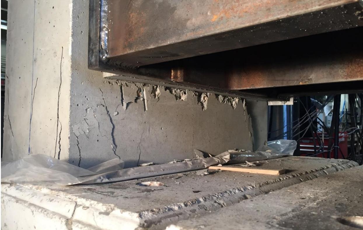
Figure 4.11 SP6-3A concrete crushing failure.
