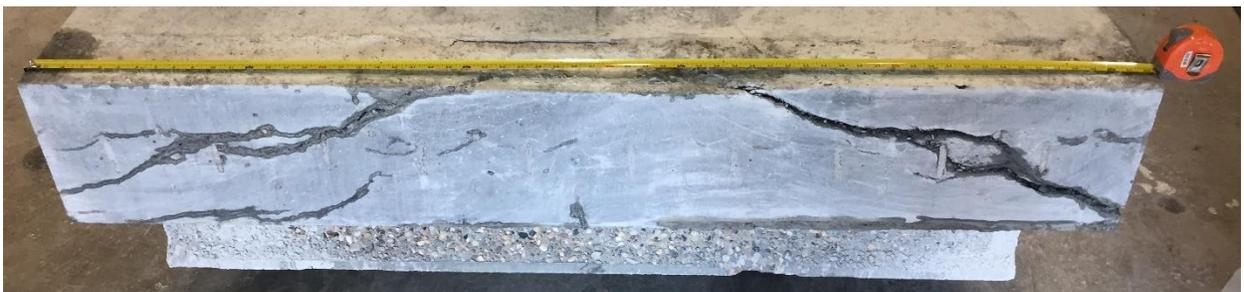
Figure 4.39 JPD deck section of north panel, cut through UHP joint (opposite cut of Figure 4.38(a), looking north).
