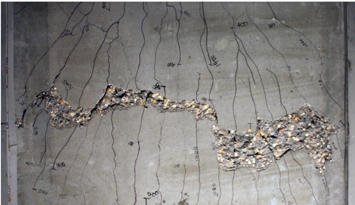
Figure 4.34 JPD failure crack after chiselling away loose pieces of concrete (south panel).
