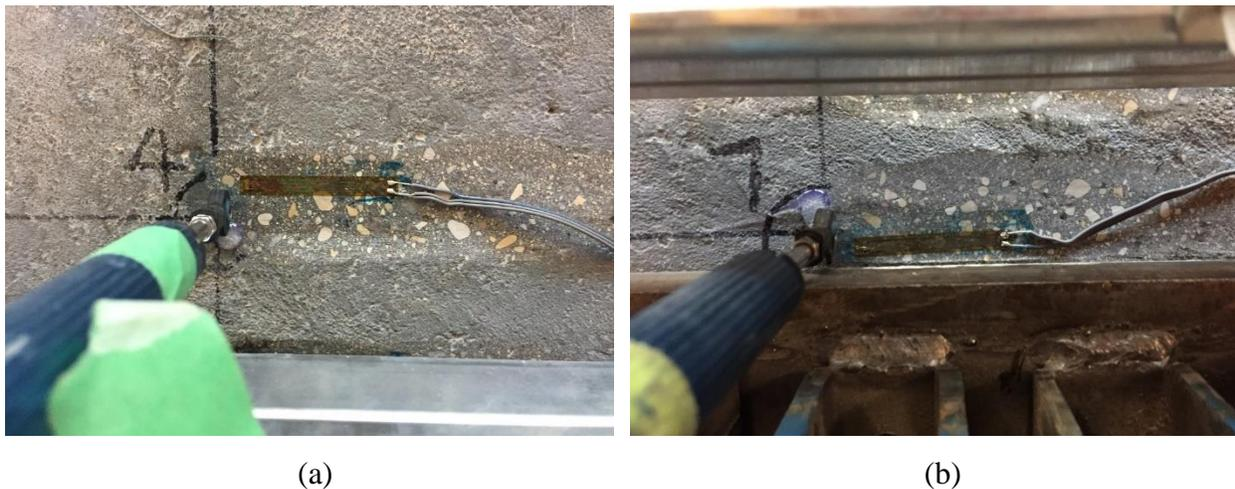
Figure 3.41 (a) CSG 1 and LVDT 4, (b) CSG 3 and LVDT 7.
