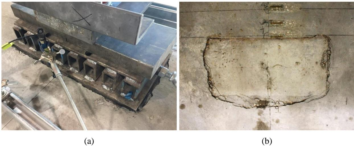
Figure 4.32 Post-failure load plate punch shape in bridge deck surface: (a) JPD with load plate; (b) FPD after load plate removed.
