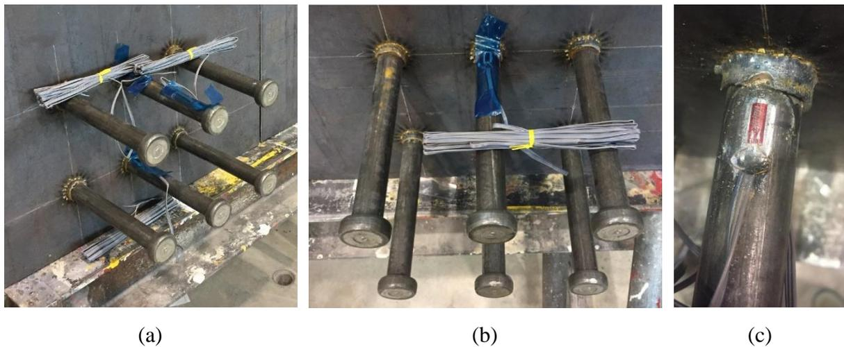
Figure 3.16 Strain gauge application.
