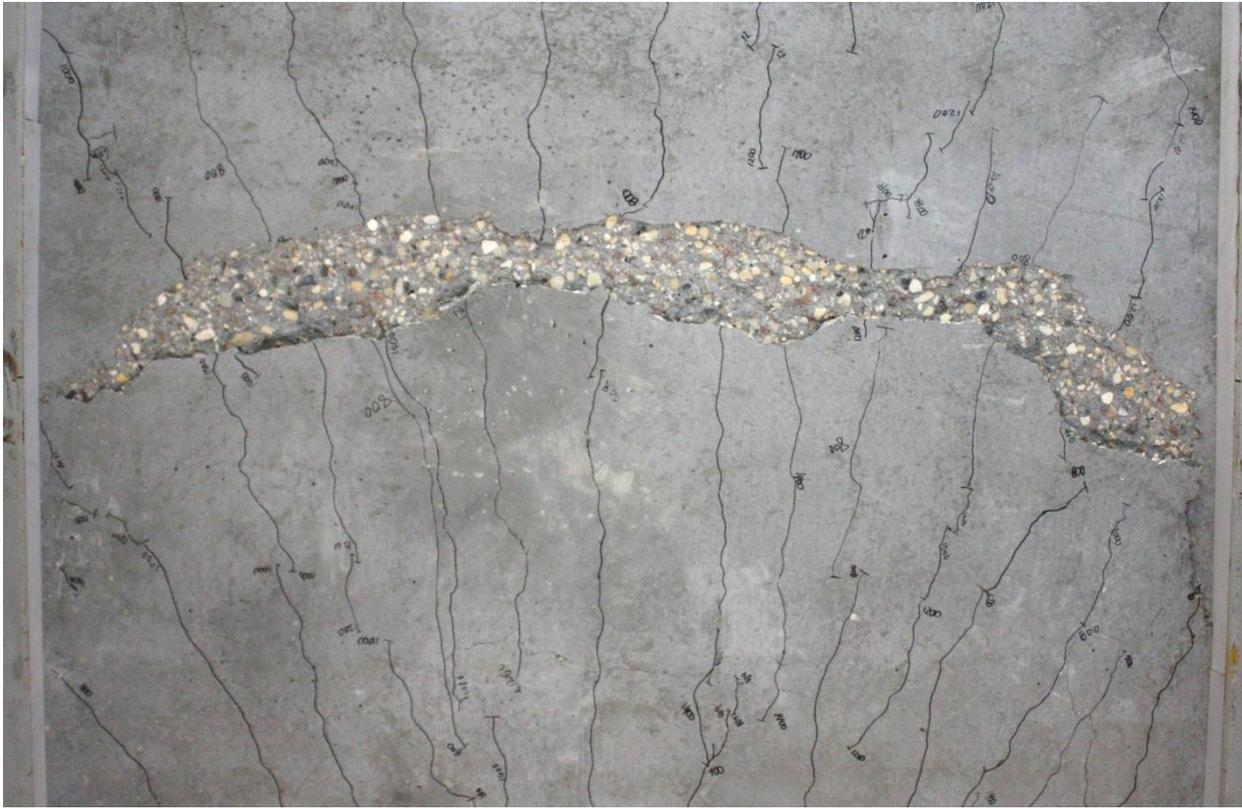
Figure 4.33 FPD failure crack after chiselling away loose pieces of concrete (north half of deck).
