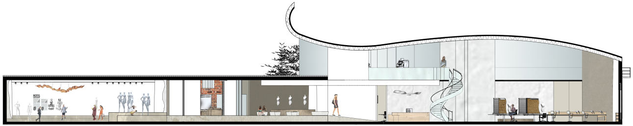
Figure 35. Interior Section: North-South Facing North. Scale: 3/16" = 1'-0"
