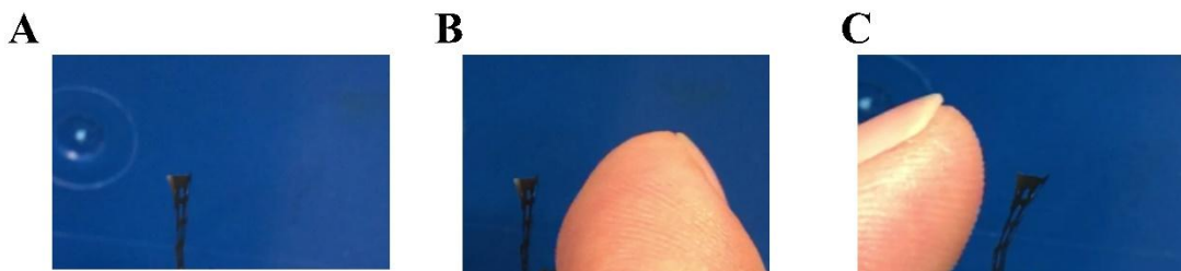
Figure 3-9 Photographs showing the actuation of DIW GO/rGO in response to human skin's humidity.
